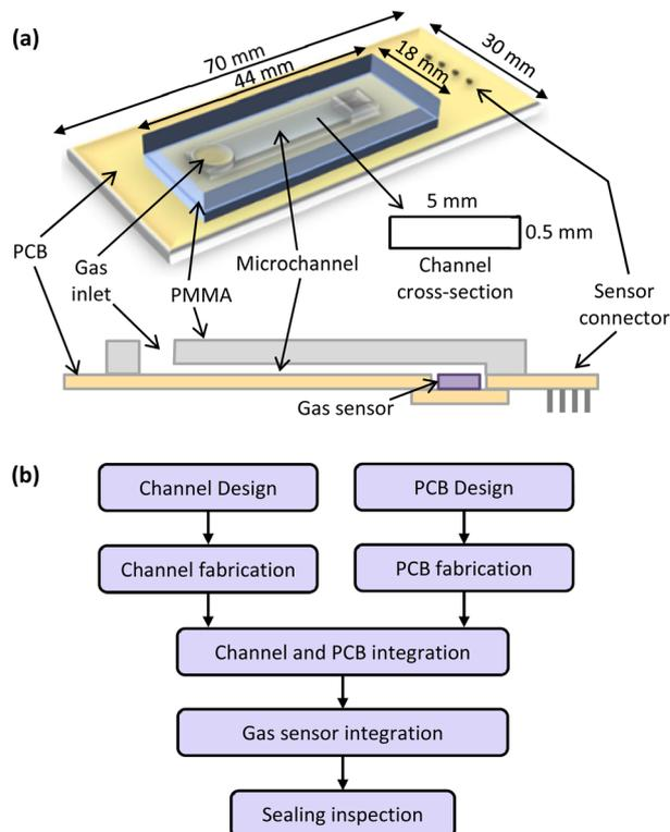
Fig. 2 Schematic design of microfluidic-based gas analyzer (a) and fabrication process of the proposed microfluidic-based PCB-PMMA gas analyzer (b).
