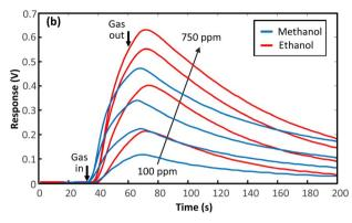
Fig. 7 (a) 3D view of the fabricated prototype 1, (b) responses for prototype 1 for various concentrations of methanol and ethanol.
