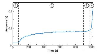
Fig. 6 Result of sealing test for gas phase for prototype made with process 8. In zone 1 inlet is open and the device is exposed to air. In zone 2 inlet closed. In zone 3 inlet is closed and the device is exposed to high concentration of ethanol vapor. In zone 4 inlet is opened.
