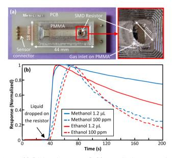
Fig. 11 (a) Fabricated prototype 5, (b) normalized responses for prototype 5 for 1.2  $\mu$ L of methanol and ethanol compared to normalized responses for prototype 1 for 100 ppm of methanol and ethanol.
