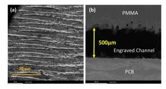
Fig. 1 The SEM images of (a) morphology of the microfluidic channel, (b) channel cross section. The scale of the micrographs is different.
