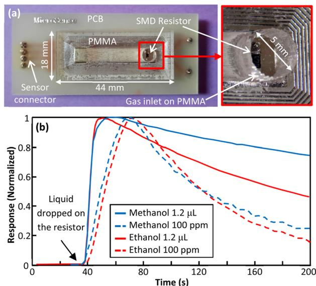
Fig. 11 (a) Fabricated prototype 5, (b) normalized responses for prototype 5 for 1.2  $\mu\text{L}$  of methanol and ethanol compared to normalized responses for prototype 1 for 100 ppm of methanol and ethanol.
