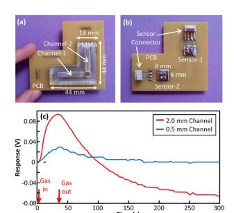
Fig. 9 (a) Fabricated prototype 3 top view, (b) fabricated prototype 3 bottom view, (c) responses of prototype 3 to 750 ppm of methanol vapor for two channel depths.
