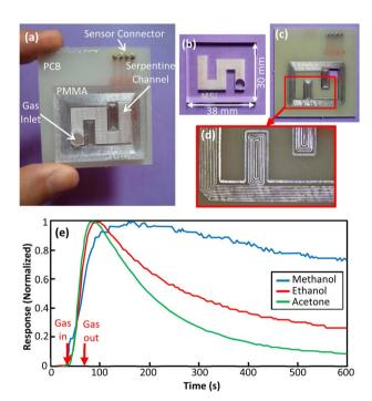
Fig. 8 (a) Fabricated prototype 2, (b) engraved serpentine channel on PMMA, (c) PCB lid, (d) zoomed view of copper pattern on PCB, (e) normalized responses for prototype 2 to 500 ppm of acetone, methanol and ethanol vapors.
