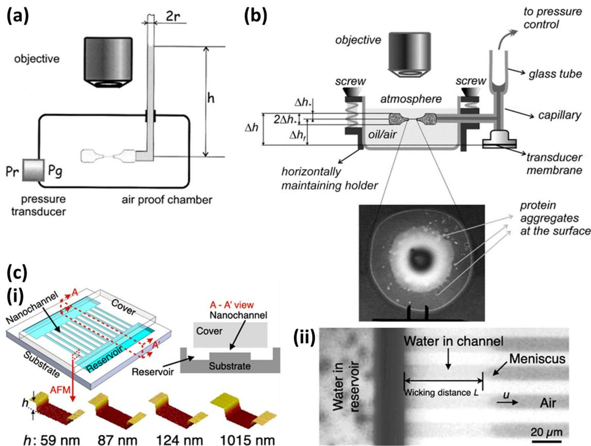
Fig. 2 Experimental setups for measuring the disjoining pressure. (a) Setup proposed by Bergeron. Reprinted with permission from (ref. 110). Copyright 2001 American Chemical Society. (b) Setup to measure disjoining pressure and thickness of film. Reprinted with permission from (ref. 111). Copyright 2004 Elsevier. (c) (i) Nanochannels with different depth and reservoirs. Reprinted with permission from (ref. 112). Copyright 2021 American Chemical Society.
