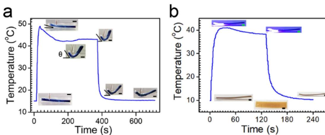
Fig. 2 (a) and (b) Temperature and bending evolutions of the hybrid hydrogel sheet with time during laser irradiation with a wavelength of 808 nm and 450 nm separately. The inserted photo images show the bending state of the sheet at different irradiation time. Scale bar: 3 mm in (a) and 2 mm in (b).
