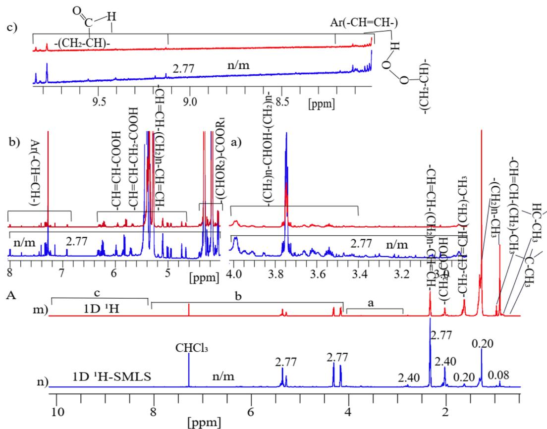
Fig. 3 (A) Typical 1D  $^1\text{H}$ -NMR full spectra from conventional (m) 1D  $^1\text{H}$  and (n)  $^1\text{H}$ -SMLS of a sample of cheese dissolved in deuterated chloroform. These spectra were divided into three sections for a clear view of spectral peaks. Sections with chemical shift regions 2.90 to 4.00 ppm (a), 4.12 to 8.00 ppm (b), and 8.01 to 9.58 ppm (c) of (A).
