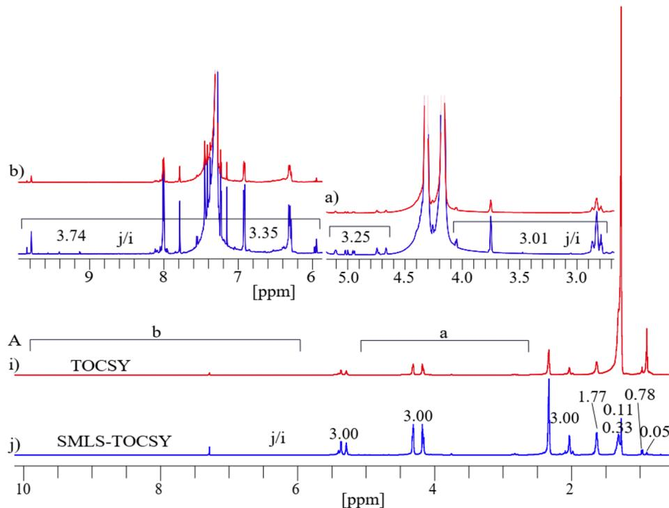
Fig. 6 (A) Projected 1D  $^1\text{H}$  spectra of (i) 2D TOCSY and (j) 2D SMLS-TOCSY in stacked spectra with the estimated numbers of the peak intensities of the butter sample. A significant sensitivity enhancement was achieved using the suppression method.
