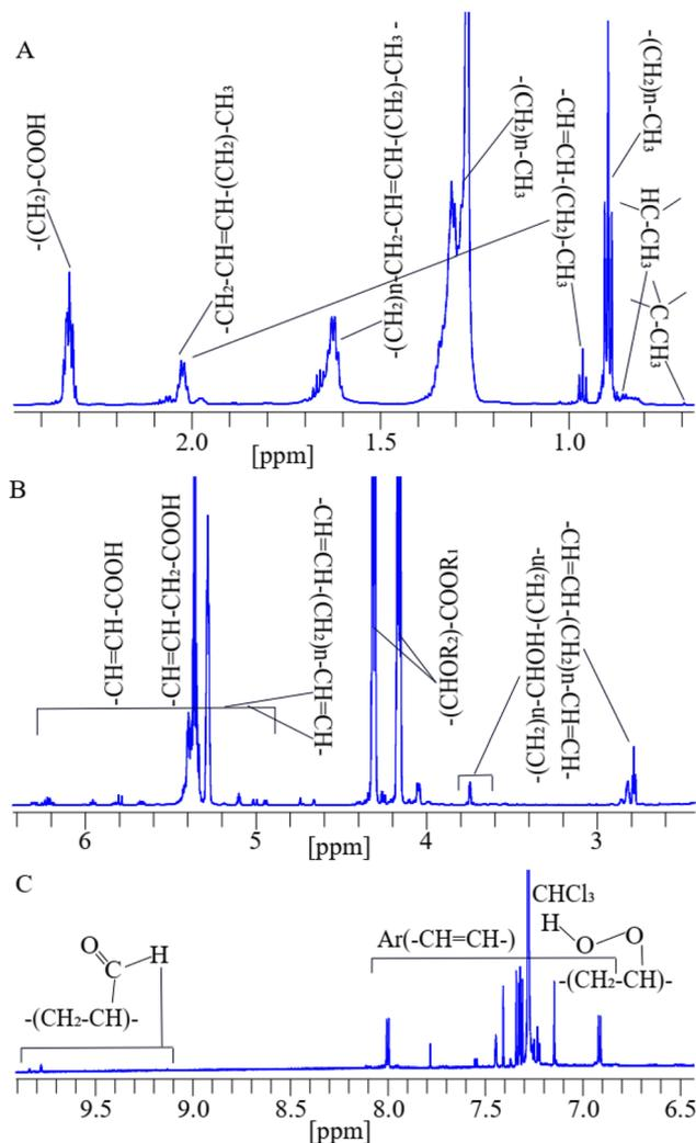
Fig. 2 A representative 1D  $^1\text{H}$ -NMR spectrum assigned with functional groups of lipids at their corresponding chemical shifts of a cheese sample dissolved in deuterated chloroform.<sup>79,80</sup>
