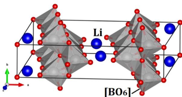
Fig. 1 Conventional representation of the hexa-metal-oxide  $\text{Li}_2\text{B}_6\text{O}_{13}$  ( $\text{B} = \text{Ti}, \text{Zr}$ ) unit cell in the  $C2/m$ . Blue balls represent the Li ions and the grey polyhedron the  $[\text{BO}_6]$  octahedron.
