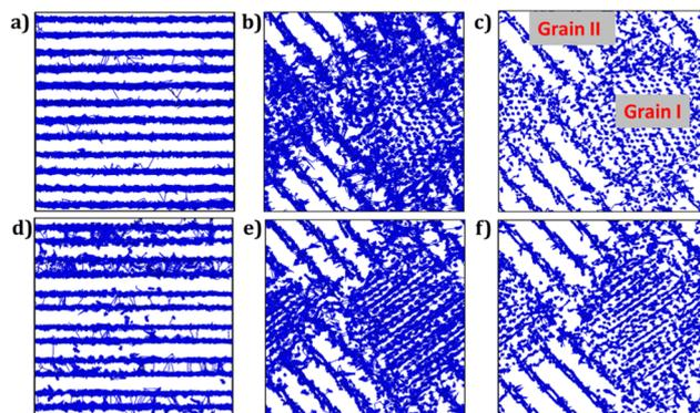
Fig. 7 Li-trajectory density maps (blue lines) of monocrystalline: (a)  $\text{Li}_2\text{Ti}_6\text{O}_{13}$ , (d) monocrystalline  $\text{Li}_2\text{Zr}_6\text{O}_{13}$ , bi-crystalline: (b)  $\text{Li}_2\text{Ti}_6\text{O}_{13}$ , (e)  $\text{Li}_2\text{Zr}_6\text{O}_{13}$  and composite: (c)  $\text{Li}_2\text{Ti}_6\text{O}_{13}@\text{Li}_2\text{Zr}_6\text{O}_{13}$ , (f)  $\text{Li}_2\text{Zr}_6\text{O}_{13}@\text{Li}_2\text{Ti}_6\text{O}_{13}$  samples.
