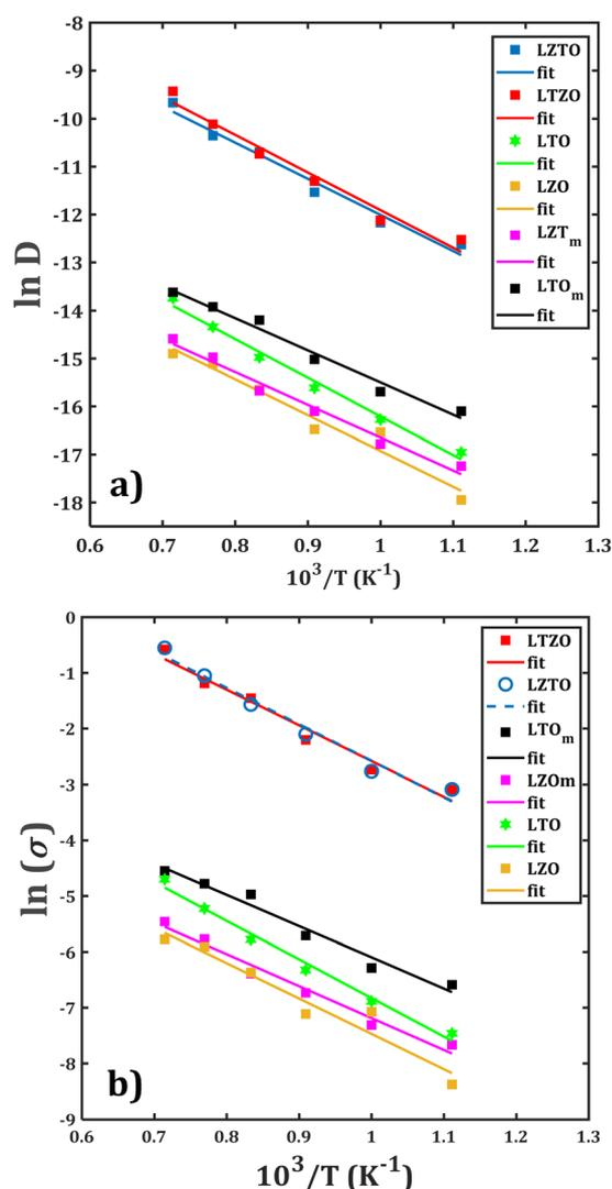
Fig. 6 Arrhenius-type dependence of (a) diffusion coefficient and (b) dc-conductivity with temperature for Li<sub>2</sub>Ti<sub>6</sub>O<sub>13</sub>/Li<sub>2</sub>Zr<sub>6</sub>O<sub>13</sub> samples: monocrystalline (LTO<sub>m</sub>/LZO<sub>m</sub>), bi-crystalline (LTO/LZO), and composite (LTZO/LZTO). In each case, the lines represent the Arrhenius fit.
