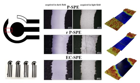
Fig. 3 Optical images, picture and 3D mapping of SPE printed on commercial PET (P-SPE), recycled PET (rP-SPE) and EC (EC-SPE).
