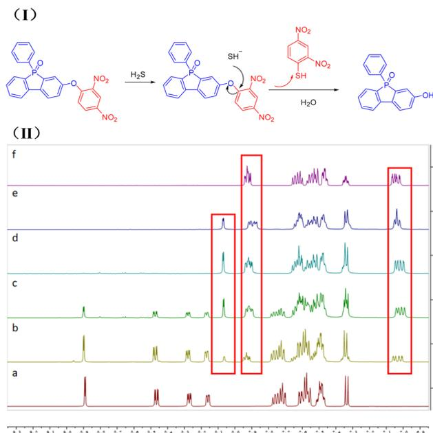
Fig. 6 (I) Possible mechanism for the probe PPF-CDNB with  $\text{H}_2\text{S}$ . (II)  $^1\text{H}$ -NMR titration experiments of probe PPF-CDNB. (a) PPF-CDNB. (b) PPF-CDNB + 1 eq. NaHS. (c) PPF-CDNB + 3 eq. NaHS. (d) PPF-CDNB + 5 eq. NaHS. (e) PPF-CDNB + 10 eq. NaHS. (f) PPF-OH.  $^1\text{H}$ -NMR measurements were performed 10 min after addition of NaHS to PPF-CDNB (600 MHz,  $\text{DMSO-d}_6$ ).
