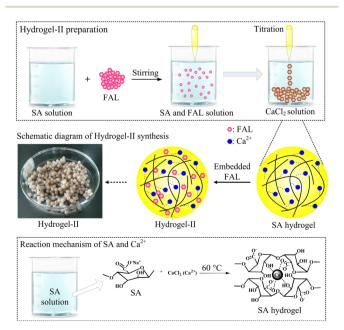
Fig. 2 Synthetic scheme of hydrogel-II and reaction mechanism.
