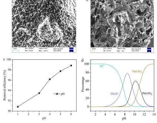
Fig. 3 (a) SEM image of hydrogel-II surface; (b) hydrogel-II planning surface; (c) solution pH impacted on Pb(II) removal efficiency; and (d) Pb(II) species at different pH values.
