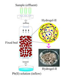
Fig. 1 The schematic diagram of fixed bed.
