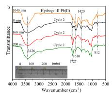
Fig. 8 FT-IR spectrum (a) second adsorption and (b) second desorption (illustrated as images of particles at different times).
