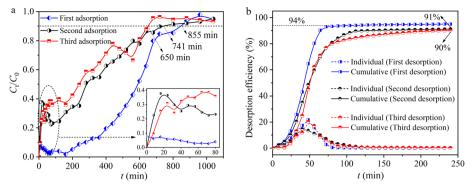
Fig. 6 Regeneration ability of hydrogel-II in a fixed bed (a) adsorption and (b) desorption.
