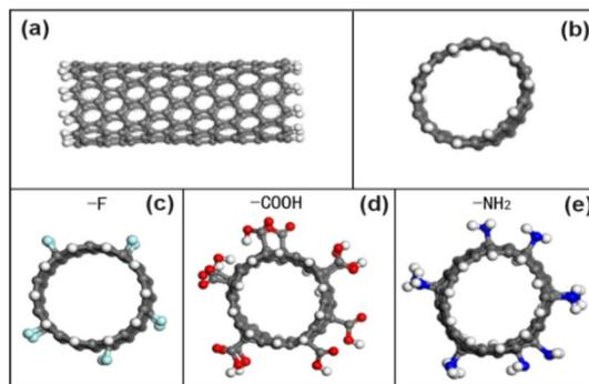
Fig. 1 (a) The side view of an unmodified CNT model; (b) the cross-sectional view of an unmodified CNT model; (c) the CNT model of grafted with F atoms; (d) the CNT model grafted with COOH groups; (e) the CNT model of grafted with NH<sub>2</sub> groups.
