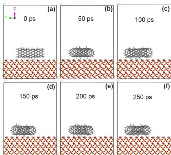
Fig. 5 State of CNT grafted with 10% fluorine groups on SiO<sub>2</sub> surface at different time. (a) 0 ps; (b) 50 ps; (c) 100 ps; (d) 150 ps; (e) 200 ps; (f) 250 ps.
