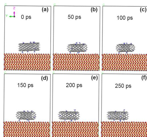
Fig. 8 State of CNT grafted with 5% amino groups on SiO<sub>2</sub> surface at different time. (a) 0 ps; (b) 50 ps; (c) 100 ps; (d) 150 ps; (e) 200 ps; (f) 250 ps.
