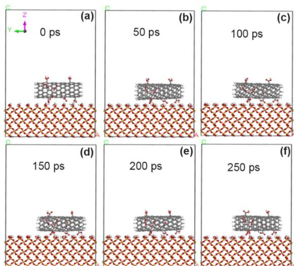
Fig. 6 State of CNT grafted with 5% carboxyl groups on SiO<sub>2</sub> surface at different time. (a) 0 ps; (b) 50 ps; (c) 100 ps; (d) 150 ps; (e) 200 ps; (f) 250 ps.
