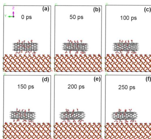
Fig. 7 State of CNT grafted with 10% carboxyl groups on SiO<sub>2</sub> surface at different time. (a) 0 ps; (b) 50 ps; (c) 100 ps; (d) 150 ps; (e) 200 ps; (f) 250 ps.
