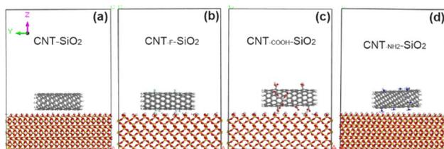
Fig. 2 Initial model of interface systems between carbon nanotubes with different functional groups and SiO<sub>2</sub>. (a) Unmodified CNT; (b) the CNT grafted with F atoms; (c) the CNT grafted with COOH groups; (d) the CNT grafted with NH<sub>2</sub> groups.
