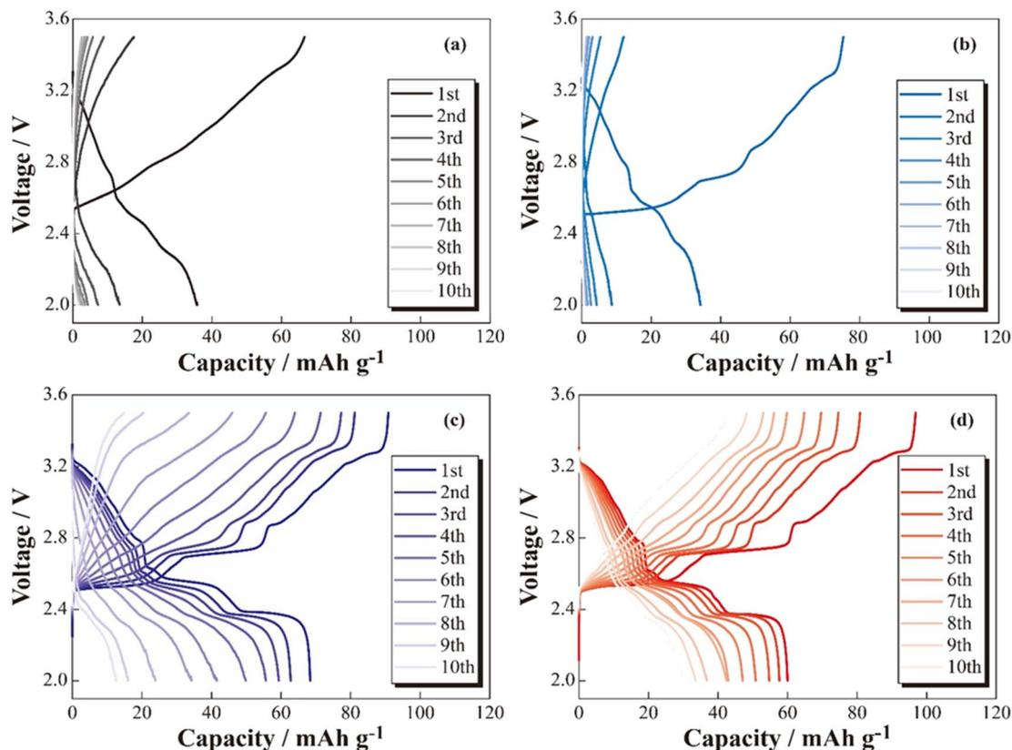
Fig. 2 Charge–discharge profiles for the [Na|SPE|NCO] (a), [Na|SPE|5 wt%  $\text{Na}_3\text{PO}_4$ -coated NCO] (b), [Na|SPE|10 wt%  $\text{Na}_3\text{PO}_4$ -coated NCO] (c) and [Na|SPE|10 wt% NZSP-coated NCO] (d) cells.
