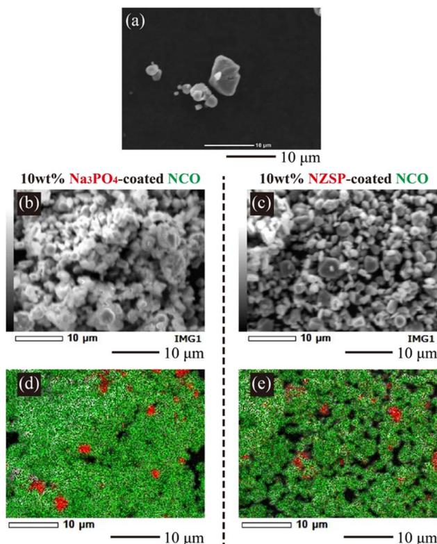
Fig. 4 SEM and EDX mapping images of the NCO powder (SEM: (a)), 10 wt% Na<sub>3</sub>PO<sub>4</sub>-coated NCO powder (SEM: (b), EDX: (d)), and 10 wt% NZSP-coated NCO powder (SEM: (c), EDX: (e)).
