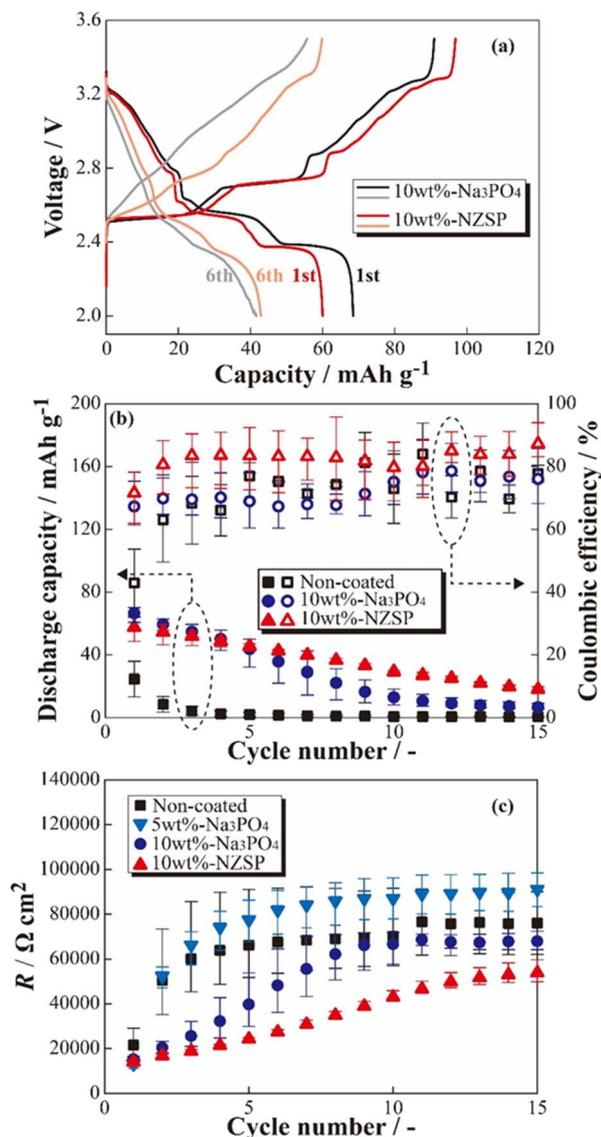
Fig. 3 Charge-discharge profiles for the [Na]SPE|10 wt% Na<sub>3</sub>PO<sub>4</sub>-coated NCO and [Na]SPE|10 wt% NZSP-coated NCO cells (a), cycle number dependences of the discharge capacity and coulombic efficiency (b), and internal resistance indexes ( $R$ ) calculated from the charge-discharge voltages (c).
