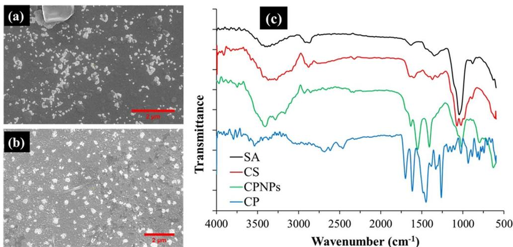
Fig. 1 SEM analyses of the, (a) blank NPs, (b) CP-NPs, and (c) FTIR spectra of SA, CS, CP, and CP-NPs.
