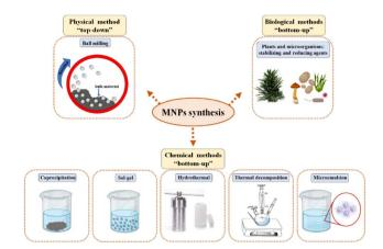
Fig. 3 Standard methods for MNP synthesis
