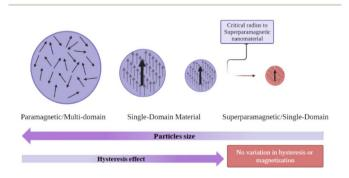
Fig. 2 Changes in the physicochemical properties of nanomaterials as a function of particle size. When particles are sized at the critical radius for superparamagnetic nanomaterials, the hysteresis and magnetization of the particle become zero.
