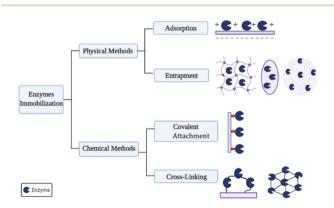
Fig. 5 Methods for enzymatic immobilization.
