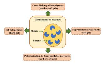
Fig. 7 The four main methods for the entrapment of enzymes out on gels.
