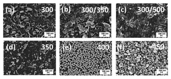
Fig. 3 Scanning electron microscopy (SEM) surface images of  $Bi_2O_3$  films. The surface of  $Bi_2O_3$  films grown at a temperature of 300 °C without annealing (a) and annealed at temperatures 350 °C (b) and 500 °C (c);  $Bi_2O_3$  films grown at temperatures 350 °C (d), 400 °C (e) and 450°(f) without annealing.
