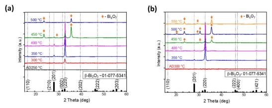
Fig. 2 XRD patterns of as-deposited (AD) at 250 °C bismuth oxide thin films and after annealing at temperatures 300–500 °C (a). XRD patterns of AD at 300 °C bismuth oxide thin films and after annealing at temperatures 350–550 °C (b).
