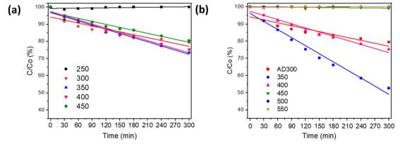
Fig. 5 Degradation curves of MO oxidation under UV-A irradiation on  $Bi_2O_3$  films prepared at different deposition temperatures (a) and deposited at 300 °C (AD) and annealed at temperatures 350–550 °C (b).
