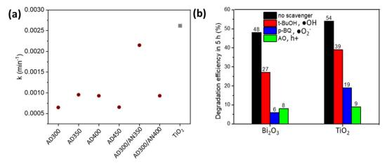
Fig. 6 Photodegradation rate constants of MO oxidation on  $Bi_2O_3$  and  $TiO_2$  thin films (a) and the influence of 'OH, ' $O_2$ ' and h<sup>+</sup> scavengers on MO degradation efficiency (b).
