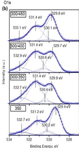
Fig. 4 X-ray photoelectron spectroscopy (XPS) spectra of Bi  $4f_{7/2}$  (a) and O 1s (b) core levels for  $Bi_2O_3$  thin films deposited and annealed at different temperatures.
