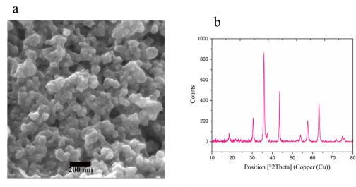
Fig. 14 FE-SEM image (a) and XRD pattern (b) of the NiFe<sub>2</sub>O<sub>4</sub>@SiO<sub>2</sub>/MgO after recycling.
