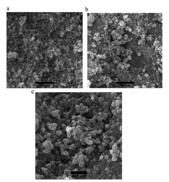
Fig. 5 FE-SEM images of the NiFe<sub>2</sub>O<sub>4</sub> (a), NiFe<sub>2</sub>O<sub>4</sub>@SiO<sub>2</sub> (b) and NiFe<sub>2</sub>O<sub>4</sub>@SiO<sub>2</sub>/MgO (c)
