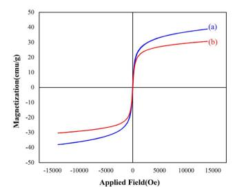
Fig. 4 The VSM analysis of NiFe<sub>2</sub>O<sub>4</sub> (a) and NiFe<sub>2</sub>O<sub>4</sub>@SiO<sub>2</sub>/MgO (b).
