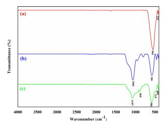
Fig. 2 The FT-IR spectra of NiFe $_2$ O $_4$  (a), NiFe $_2$ O $_4$ @SiO $_2$  (b), and NiFe $_2$ O $_4$ @SiO $_2$ /MgO (c).
