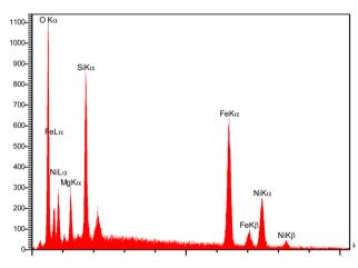
Fig. 7 EDS spectrum of the NiFe<sub>2</sub>O<sub>4</sub>@SiO<sub>2</sub>/MgO
