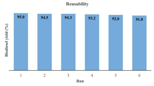
Fig. 13 The reusability of the NiFe<sub>2</sub>O<sub>4</sub>@SiO<sub>2</sub>/MgO under optimized reaction condition.
