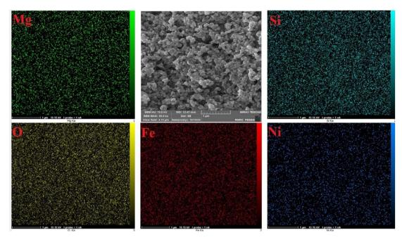
Fig. 8 Picture of the elemental mapping of the NiFe<sub>2</sub>O<sub>4</sub>@SiO<sub>2</sub>/MgO
