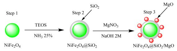
Fig. 1 Stepwise preparation of NiFe<sub>2</sub>O<sub>4</sub>@SiO<sub>2</sub>/MgO core-shell magnetic nano-catalyst.
