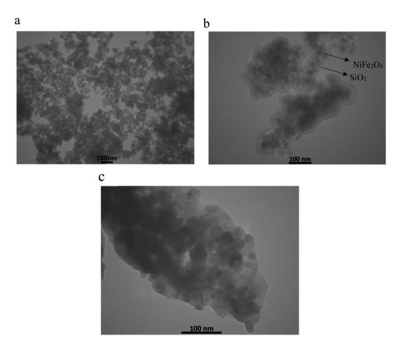
Fig. 6 TEM images of the NiFe<sub>2</sub>O<sub>4</sub> (a), NiFe<sub>2</sub>O<sub>4</sub>@SiO<sub>2</sub> (b) and NiFe<sub>2</sub>O<sub>4</sub>@SiO<sub>2</sub>/MgO (c).
