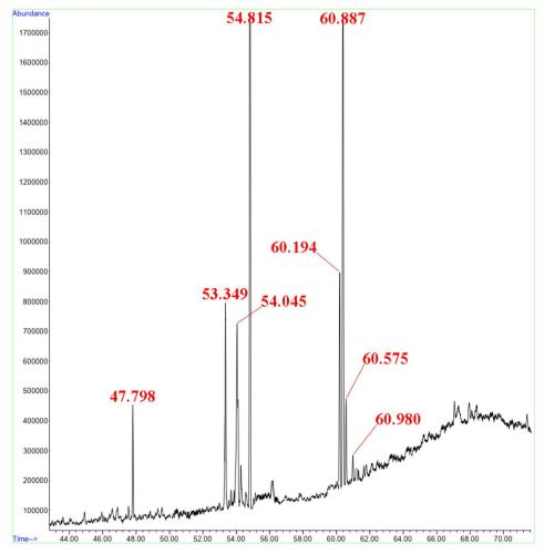
Fig. 12 GC-MS spectrum of Scenedesmus sp. biodiesel synthesized under optimum conditions.
