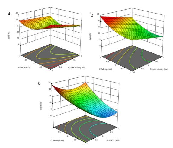
Fig. 10 The response surface plots: (a) interactive effect of light intensity and  $NO_3$  concentration, (b) interactive effect of light intensity and salinity concentration, (c) interactive effect of  $NO_3$  concentration and salinity concentration.
