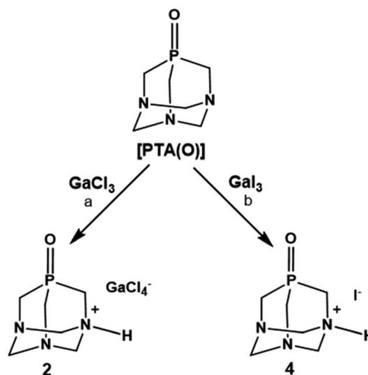
**Scheme 2** Products of reactions of [PTA(O)] with GaCl<sub>3</sub> and GaI<sub>3</sub>. Reaction conditions: (a) [Ga] : [P(O)] = 1 : 1.2; DCM@rt; or MeOH/DCM@rt. (b) [Ga] : [P(O)] = 1 : 1.2; H<sub>2</sub>O@rt; or DCM@rt.
