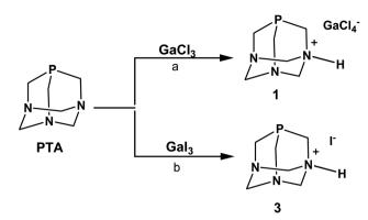
Scheme 1 Products of reactions of PTA with GaCl $_3$  and Gal $_3$ . Reaction conditions: (a) [Ga]:[P] = 1:1.2; DCM@rt; or DCM@0 °C; or DCM/Et $_3$ N@rt. (b) [Ga]:[P] = 1:1.2; EtOAc@rt; or Et $_2$ O@rt; or solid state reaction.
