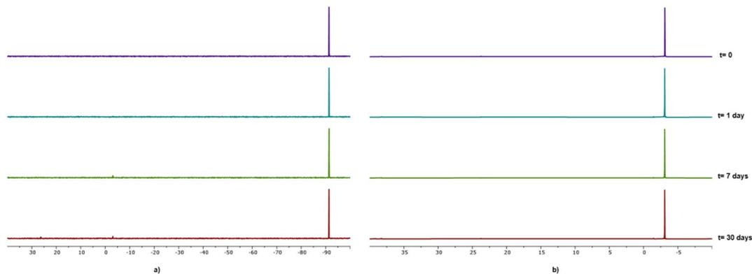
Fig. 5  $^{31}\text{P}\{^1\text{H}\}$  NMR spectra of  $\text{D}_2\text{O}$  solutions (0.025 M) of [PTA-H]·[GaCl<sub>4</sub>] **1** (a) and [PTA(O)-H]·[GaCl<sub>4</sub>] **2** (b) recorded at several times. The spectra were recorded with a transmitter frequency offset of  $-40$  ppm and a spectral width of 200 ppm. Spectral widths shown in the figure were expanded in the region where signals were detected. Each spectrum was normalised to the tallest peak intensity.
