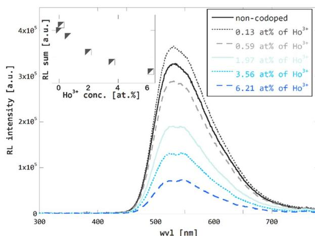
**Fig. 6** Radioluminescence (40 kV, 15 mA X-rays) spectra of non-codoped GGAG:Ce and Ho<sup>3+</sup> codoped GGAG:Ce. Radioluminescence spectra integrals plotted against Ho<sup>3+</sup> codopant concentration in the inset.
