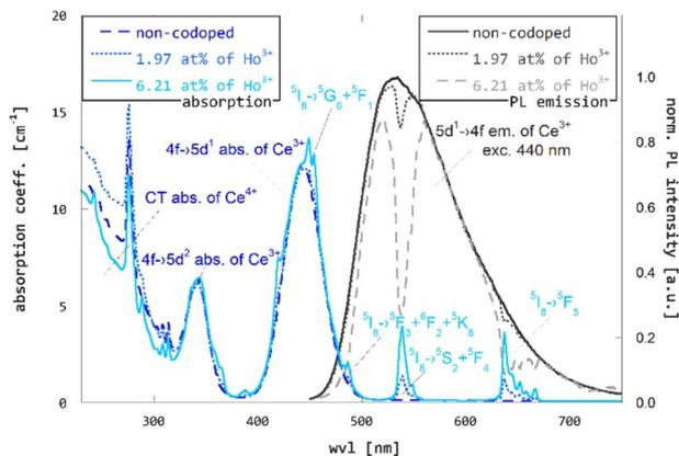
Fig. 3 Photoluminescence (excitation to 440 nm) and absorption spectra of non-codoped GGAG:Ce and Ho<sup>3+</sup> codoped GGAG:Ce shows the spectral overlap.
