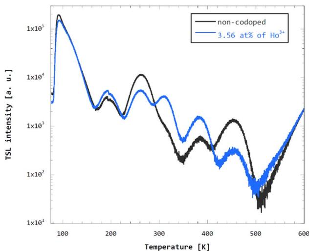
Fig. 8 Spectrally unresolved TSL glow curves of non-codoped and  $\text{Ho}^{3+}$  codoped GGAG:Ce measured after 10 minutes of irradiation with 40 kV/15 mA X-rays at 77 K and  $0.1 \text{ K s}^{-1}$  heating rate.
