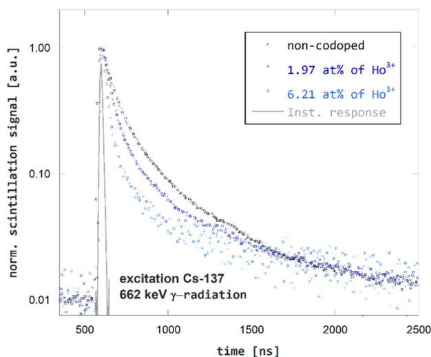
**Fig. 5** Scintillation decay kinetics of non-codoped GGAG:Ce and Ho<sup>3+</sup> codoped GGAG:Ce excited by <sup>137</sup>Cs  $\gamma$ -radiation.
