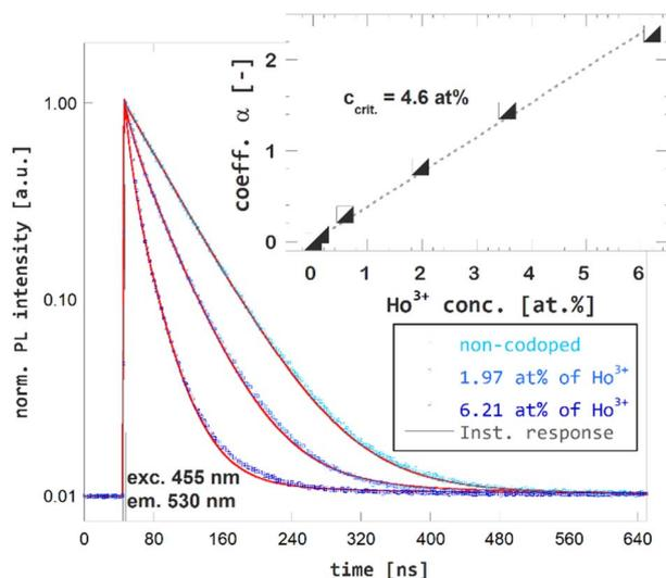
Fig. 4 Photoluminescence decay kinetics of Ce<sup>3+</sup> (excitation 455 nm, emission 530 nm) in non-codoped GGAG:Ce and Ho<sup>3+</sup> codoped GGAG:Ce. The red lines show the IH model fit of the data.
