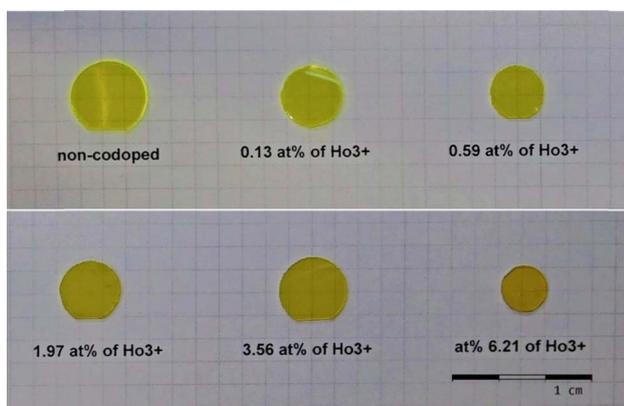
Fig. 2 Photography of GGAG:Ce crystals codoped with various concentrations of Ho<sup>3+</sup>. The reddish tint is due to Ho<sup>3+</sup> codoping of the crystals.
