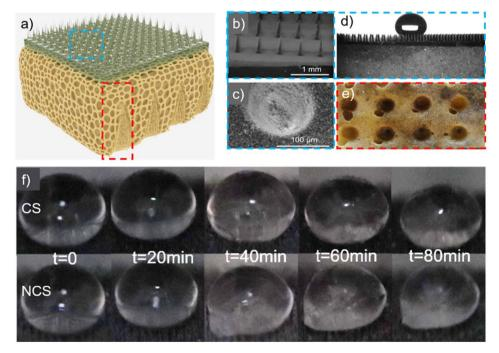
Fig. 3 (a) Sketch of the sample topography. (b and c) SEM images of the surface topography. Nano-rods with a length and diameter of 3  $\mu$ m and 100 nm were observed. (d) Superhydrophobic state of the droplet on the surface. (e) Back details of the sample. (f) Delay in the icing process. The water content of the prepared samples was 1.96%.
