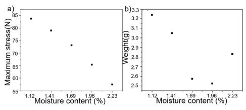
Fig. 6 (a) Maximum tensile stress with different water contents. (b) The mass of the same volume with different water contents.
