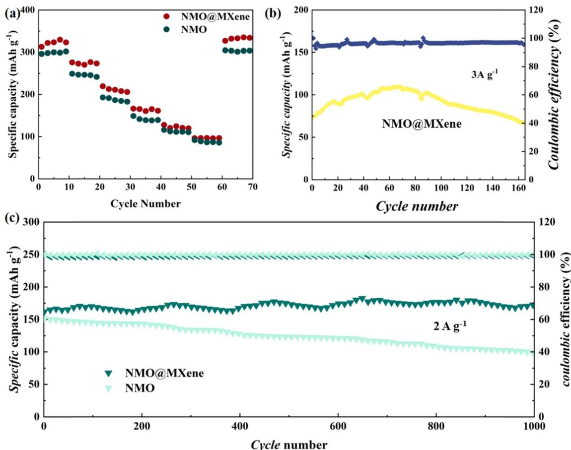
Fig. 6 (a) Rate performances of ZIBs with NMO@MXene and NMO; cycling performance at 3 A g<sup>-1</sup> (b), and long-term cycling performance at 2.0 A g<sup>-1</sup> (c) of the ZIBs with NMO@MXene and NMO.
