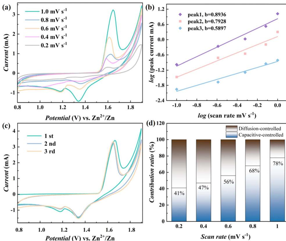
Fig. 4 (a) CV curves of the ZIBs with NMO@MXene at various scan rates; (b) determination of the  $b$  value according to  $\log i$  and  $\log v$  plots; (c) CV curves of the ZIBs with NMO@MXene at  $0.2 \text{ mV s}^{-1}$ ; (d) contribution ratios of capacitive-like and diffusion-controlled processes at different scan rates.
