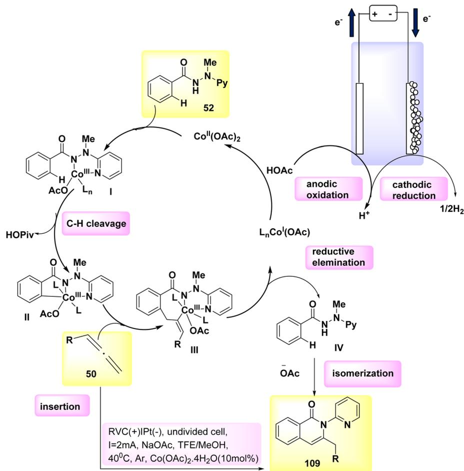
Scheme 41 Electrochemical synthesis of carbon–H<sub>2</sub> annulation product **109** with its proposed mechanism.
