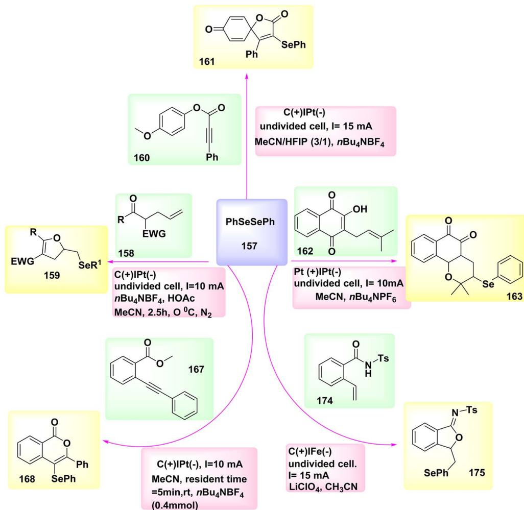
Scheme 60 Electrochemical synthesis of substituted selenated dihydrofuran 159, 3-selenated spiro[4.5]trienones 161, selenium-containing naphthoquinones 163, isocoumarin 168, and selenatedisobenzofuran 175.
