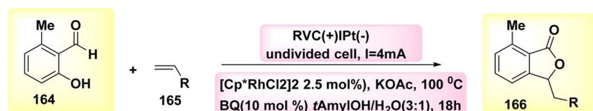
Scheme 64 Electrosynthesis of substituted isobenzofuran-1(3H)-one 166.
