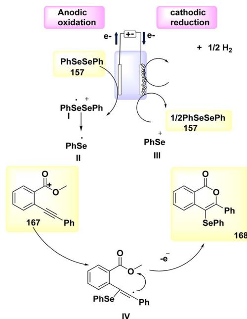
Scheme 65 Mechanism of formation of isocoumarin 168.
