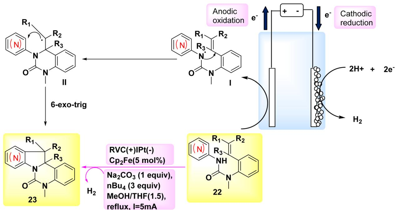
Scheme 8 Electrochemical synthesis of azaindolines 23 with its proposed mechanism.
