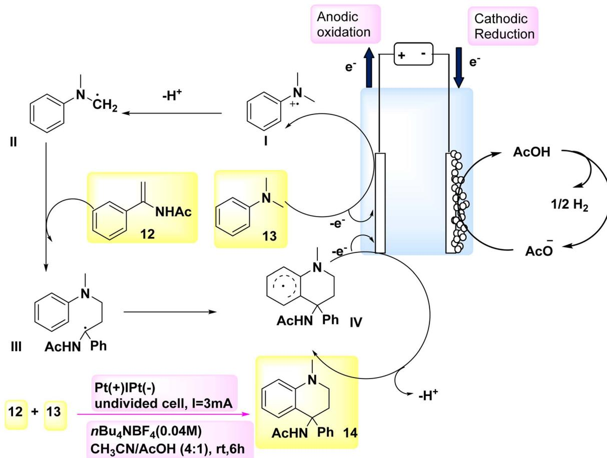
Scheme 5 Electrochemical synthesis of *N*-(1-methyl-4-phenyl-1,2,3,4-tetrahydro-quinolin-4-yl)acetamide **14** with its proposed mechanism.
