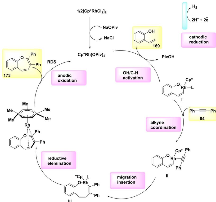
Scheme 68 Electrosynthesis of benzoxepine 173 with its proposed mechanism.
