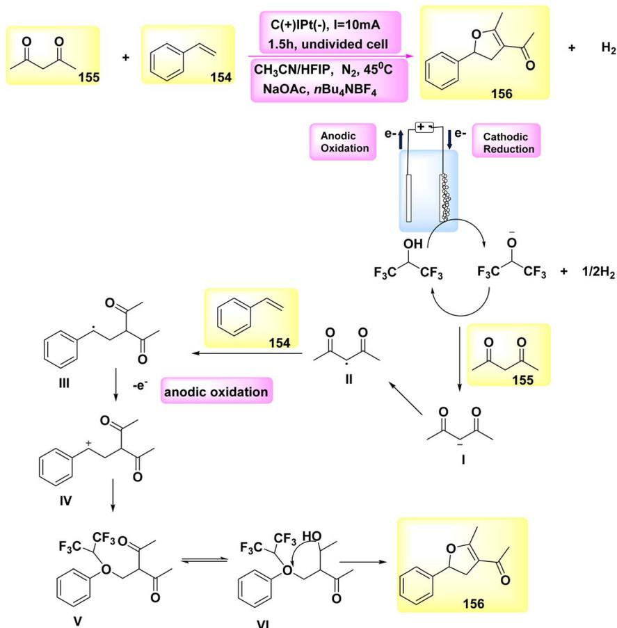
Scheme 59 Electrochemical synthesis of substituted dihydrofuran **156** with its mechanism.
