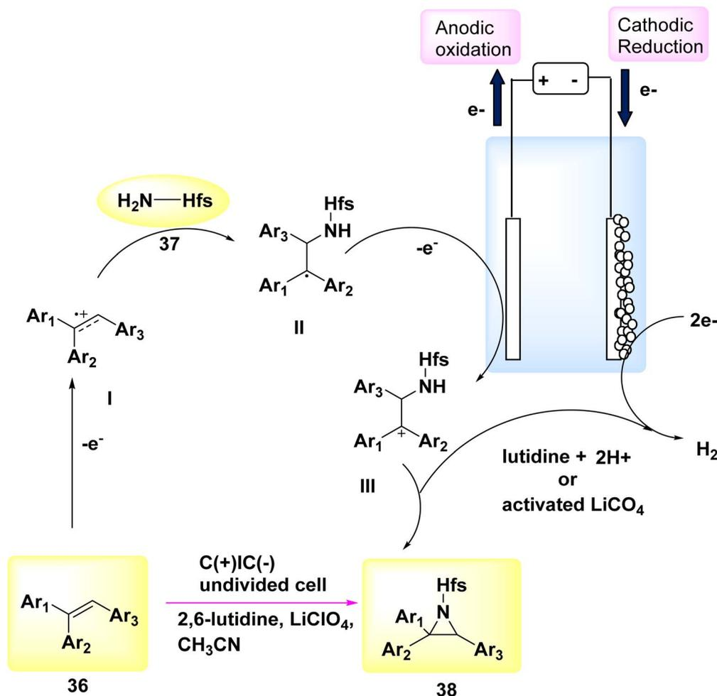
Scheme 14 Electrochemical synthesis of aziridine 38 with its proposed mechanism.
