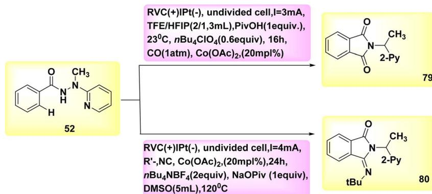
Scheme 28 Electrochemical synthesis of substituted cyclic imidates 79 and 80.
