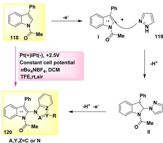
Scheme 48 Electrochemical synthesis of 2-heteroaryl- $C_{16}H_{13}NO$  **120** with proposed mechanism.
