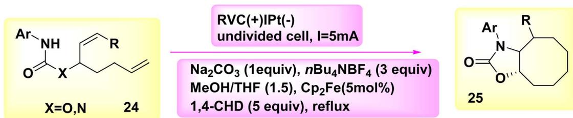
Scheme 9 Electrosynthesis of 7 membered functionalized carbocycles 25.
