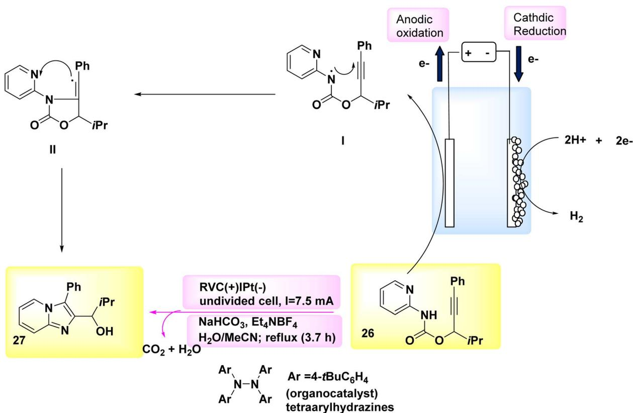
Scheme 10 Electrochemical synthesis of fused imidazo-pyridine 27 with its proposed mechanism.
