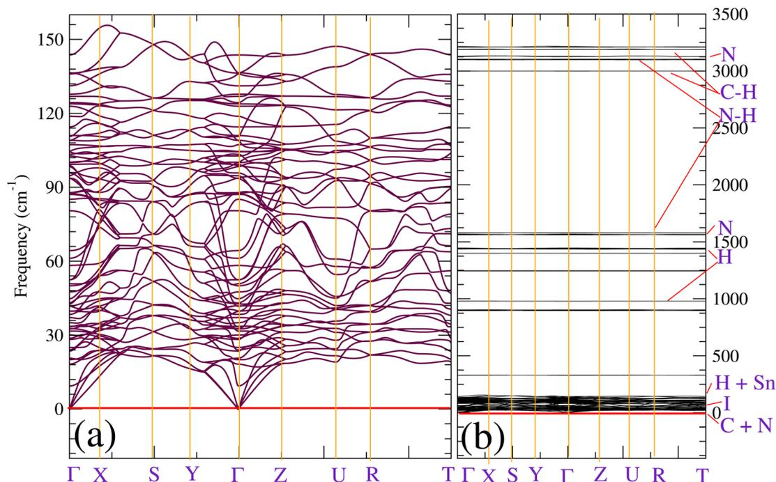
**Fig. 1** (Color online) Phonon dispersion of orthorhombic  $\text{CH}_3\text{NH}_3\text{SnI}_3$ . The plots (a) and (b) represent a zoom for frequencies from 0 to  $200\text{ cm}^{-1}$  and the full phonon spectra, respectively. Atoms whose vibrations are associated with the different modes are indicated in (b).
