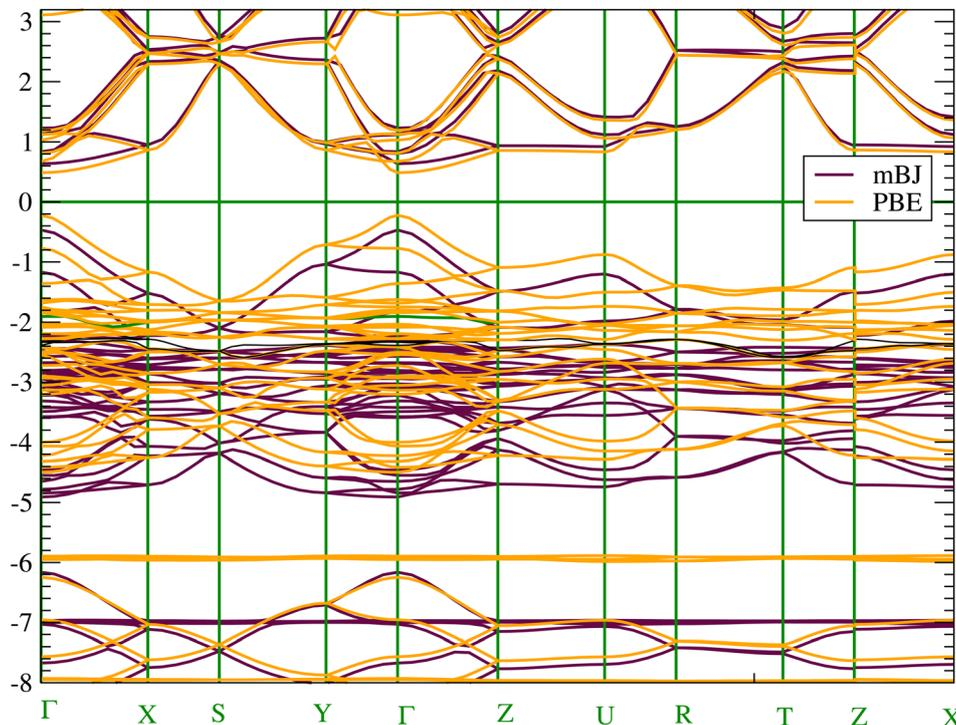
Fig. 3 (Color online) Electronic band structure of  $\text{CH}_3\text{NH}_3\text{SnI}_3$  calculated with (a) at mBJ-GGA and (b) PBE-GGA.
