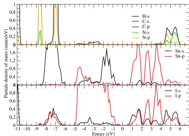
Fig. 4 Partial electronic density of states of un-strained  $\text{CH}_3\text{NH}_3\text{SnI}_3$ . The PDOS provides valuable insights into the contributions of specific atoms and orbitals to the electronic structure of the investigated structure.
