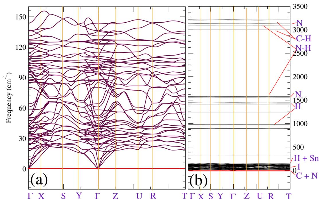
**Fig. 1** (Color online) Phonon dispersion of orthorhombic  $\text{CH}_3\text{NH}_3\text{SnI}_3$ . The plots (a) and (b) represent a zoom for frequencies from 0 to  $200\text{ cm}^{-1}$  and the full phonon spectra, respectively. Atoms whose vibrations are associated with the different modes are indicated in (b).
