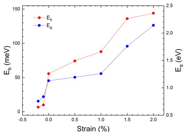
Fig. 5 The evolution of band gap and binding energy as a function of strain. In this plot, the Wannier-Mott Model is used to calculate the exciton binding energy  $E_b$ . The exciton energy ( $E_{\text{exciton}}$ ) can be approximated by:  $E_{\text{exciton}} = E_g - E_b$ .
