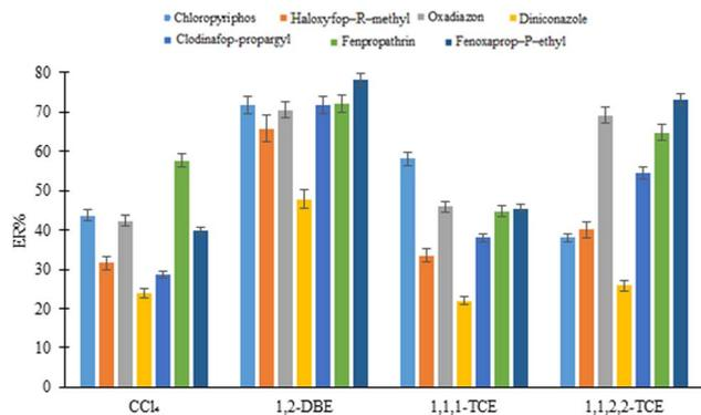
Fig. 5 Selection of extraction solvent in DLLME. Extraction conditions: are the same as those used in Fig. 4(b), except 5.0%, w/v, NaCl was dissolved in the DLLME aqueous phase.
