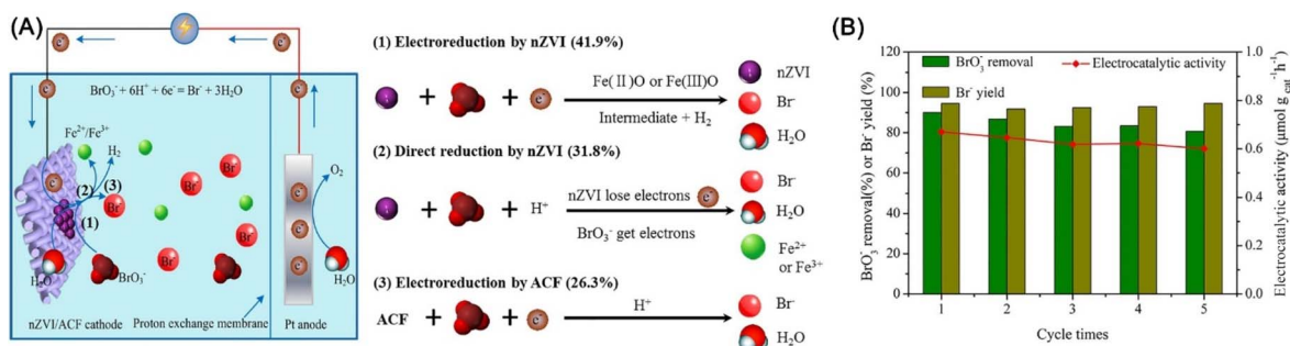
Fig. 19 (A) Mechanism of electrocatalytic BrO 3 - reduction by nZVI/ACF; (B) electrocatalytic reduction performance of BrO 3 - during five cycles, 134 copyright 2020 Elsevier.
