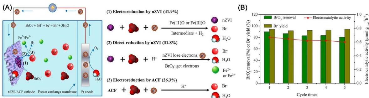
Fig. 19 (A) Mechanism of electrocatalytic BrO<sub>3</sub><sup>-</sup> reduction by nZVI/ACF; (B) electrocatalytic reduction performance of BrO<sub>3</sub><sup>-</sup> during five cycles,<sup>134</sup> copyright 2020 Elsevier.
