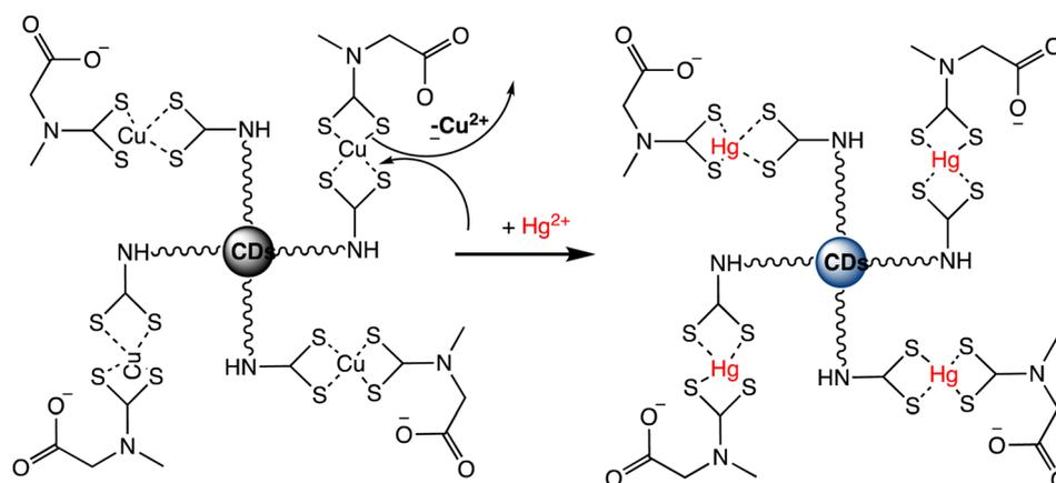
Scheme 7 Fluorescent "Turn On" nanosensor for surface-bound CuDTC2 complex Hg(II) detection based on Cu(II) displacement due to Hg(II).
