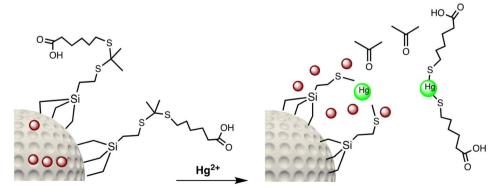
Scheme 13 Graphic for Hg(II) ions detection mechanism.
