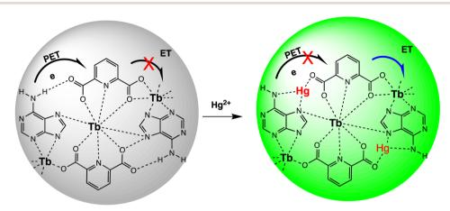
Scheme 23 Graphic representation of Hg(II) sensing using Ad/Tb/DPA via PET.
