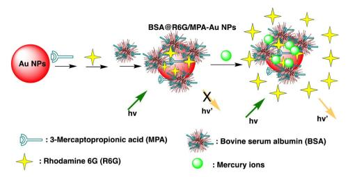
Scheme 3 Schematic of BSA@R6G/MPA-Au NP preparation and Hg(II) ions sensing
