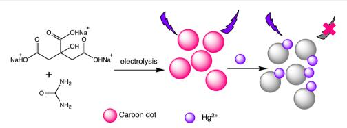
Scheme 8 Graphic for Hg(II) and Cys detection via the carbon dots
