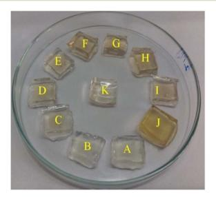
Fig. 5 Color changes of hydrogel with Hg(ii) ions (0–20 minutes) (reproduced from ref. 61 with permission from Elsevier Ltd, Copyright © 2016).
