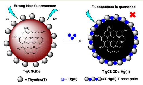
Scheme 10 Schematic representation of Hg(II) binding on T-qCNQDs surface
