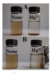
Fig. 15 Separation of Hg<sup>2+</sup>-bound nano sensor from aqueous via using a magnet (A) before apply a magnet and (B) after apply a magnet for separation (reproduced from ref. 134 with permission from Elsevier Inc, Copyright © 2012).
