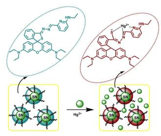
Scheme 11 Schematic illustration of Hg(||) binding with rhodamine-functionalized silica nanoparticles (RFSNP).
