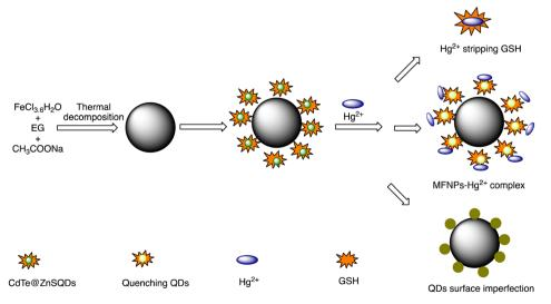
Scheme 16 Schematic illustration for interaction of MFNPs with Hq(II).
