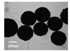
Fig. 8 SEM and TEM mages of as prepared  $Fe_3O_4$ @AgNPS (reproduced from ref. 64, with permission from Royal Society of Chemistry, Copyright @ 2017).
