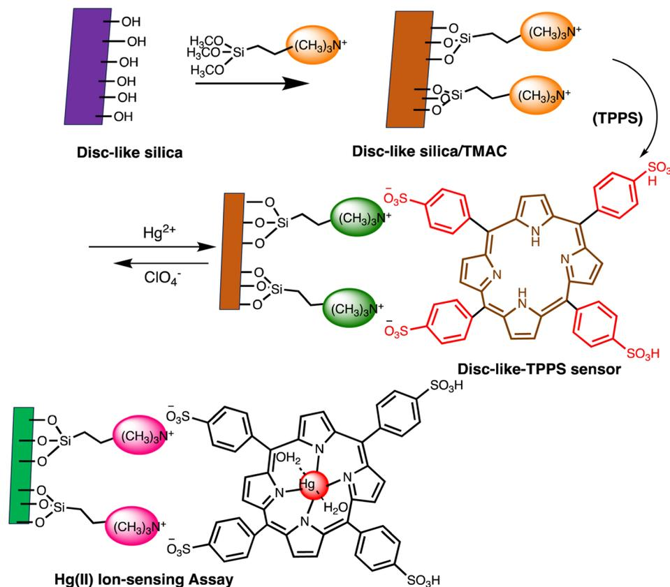
Scheme 14 Schematic representation of disc-like-TPPS sensor preparation and Hg(II) sensing.
