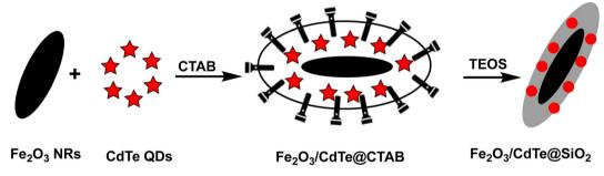
Scheme 18 Graphic for CdTe/Fe<sub>2</sub>O<sub>3</sub>@SiO<sub>2</sub>NPS preparation.
