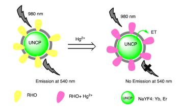
Scheme 12 Graphic for luminescence resonance energy transfer between NaYF4:Yb, Er UCNPs and the probe RHO for  $Hg(\shortparallel)$  ion sensing.
