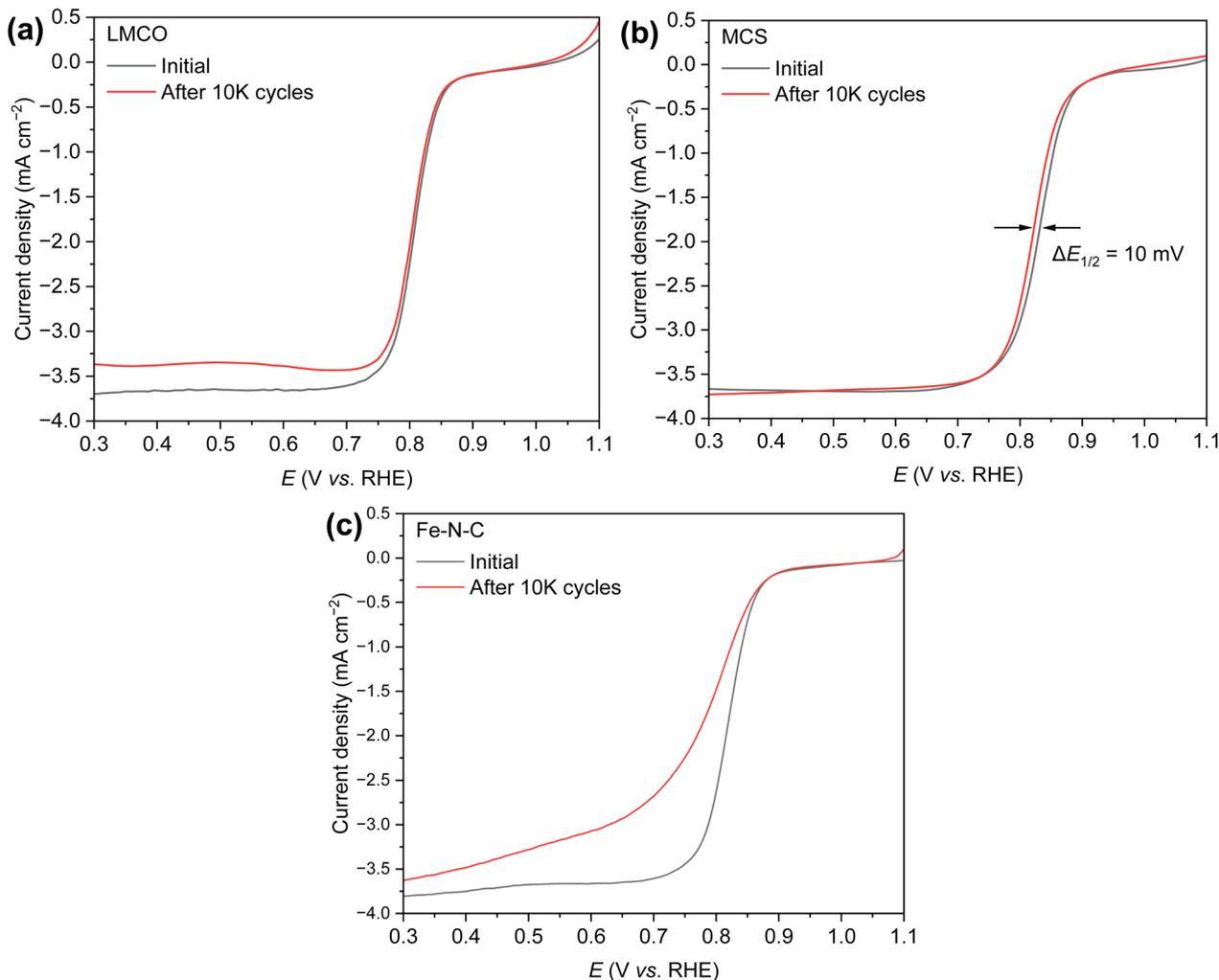
Fig. 5 ORR polarization curves of (a) LMCO, (b) MCS, and (c) Fe-N-C before and after 10k ADT cycles in O<sub>2</sub>-saturated 1 M KOH + 10 mM NaBH<sub>4</sub> solution at 25 °C and 1600 rpm.
