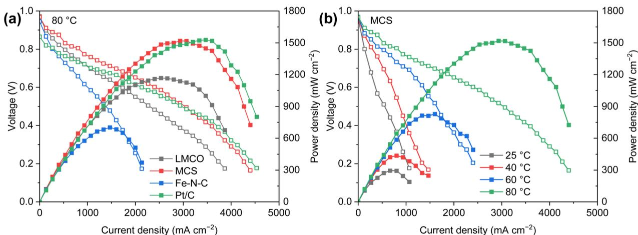
Fig. 7 DBFC polarization and corresponding power density curves of (a) various cathode catalysts measured at  $80^\circ \text{C}$ , and (b) MCS cathode measured at  $25$ – $80^\circ \text{C}$ . Anode:  $0.15 \text{ mg}_{\text{Pt}} \text{ cm}^{-2}$  40% Pt/C; membrane:  $15 \mu\text{m}$  Alkymer® W-211415; cathode:  $1.5 \text{ mg}_{\text{catalyst}} \text{ cm}^{-2}$ .
