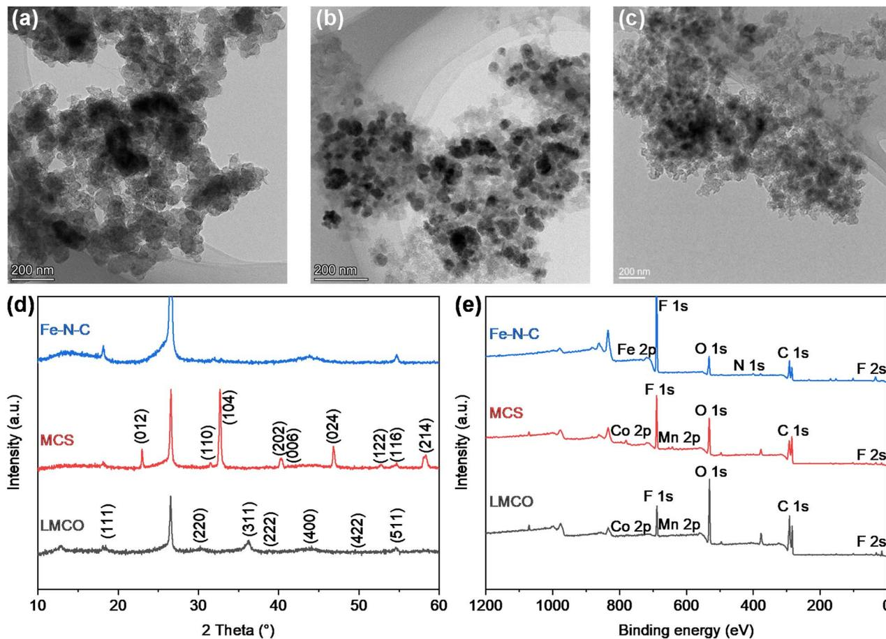
Fig. 9 TEM images of (a) LMCO, (b) MCS, and (c) Fe-N-C, (d) XRD patterns, and (e) XPS survey spectra after durability tests.
