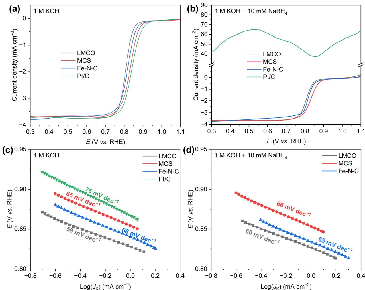
Fig. 3 ORR polarization curves of various catalysts in (a) 1 M KOH and (b) 1 M KOH + 10 mM NaBH<sub>4</sub>; Tafel plots of various catalysts in (c) 1 M KOH and (d) 1 M KOH + 10 mM NaBH<sub>4</sub>.
