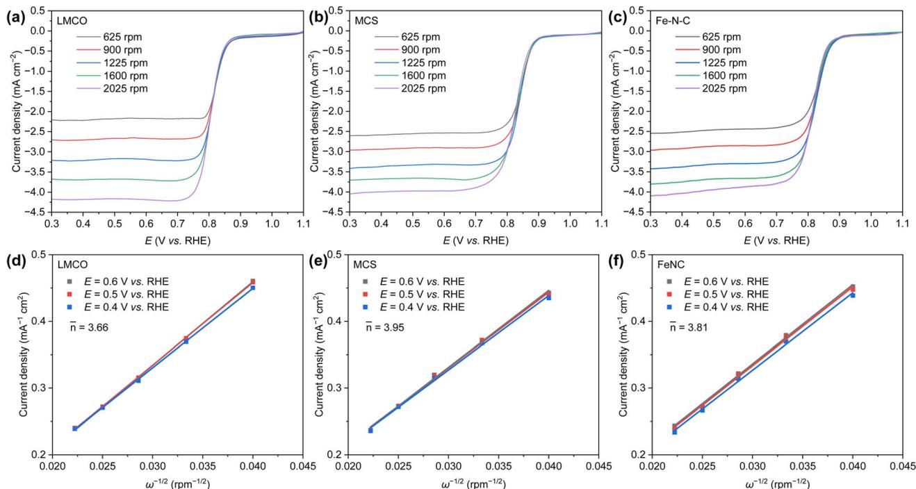
Fig. 4 ORR polarization curves of (a) LMCO, (b) MCS, and (c) Fe-N-C in  $O_2$ -saturated 1 M KOH solution at a sweep rate of  $20 \text{ mV s}^{-1}$  with different rotation speed (400–2025 rpm); the related Koutecky–Levich plots of (d) LMCO, (e) MCS, and (f) Fe-N-C at different electrode potentials.
