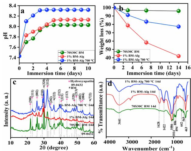
Fig. 3 (a) Changes observed in pH values up to 10 days of immersion of 70S30C BM, 1% BM-Alg, and 1% BM-Alg 700 °C composite in SBF as a function of time. (b) Weight loss percentage of 70S30C BM, 1% BM-Alg, and 1% BM-Alg 700 °C pellet after 3, 7, and 14 days of immersion in SBF. (c) Representative XRD and (d) FTIR spectra of 70S30C BM, 1% BM-Alg, and 1% BM-Alg 700 °C after 14 days of *in vitro* bioactivity study.
