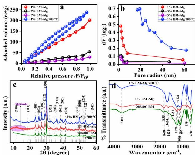
Fig. 1 (a) BET (surface area analysis). (b) BJH (pore size distribution) of 1% (red curve), 3% (black curve), 5% (purple curve) BM–Alg, and 1% BM–Alg 700 °C (blue curve). (c) XRD and (d) FTIR analysis of 70S30C BM, 1% BM–Alg, and 1% BM–Alg 700 °C composite.
