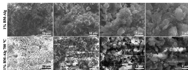
Fig. 2 SEM images of 1% BM–Alg and 1% BM–Alg 700 °C composite at different magnification.
