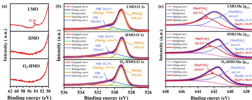
Fig. 5 The XPS fitted splitting for LMO, HMO and O<sub>3</sub>-HMO: (a) Li 1s, (b) O 1s, (c) Mn 2p<sub>3/2</sub>.
