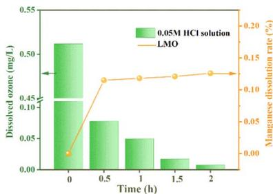
Fig. 7 Dissolved O<sub>3</sub> concentration and MDL after adding LMO.
