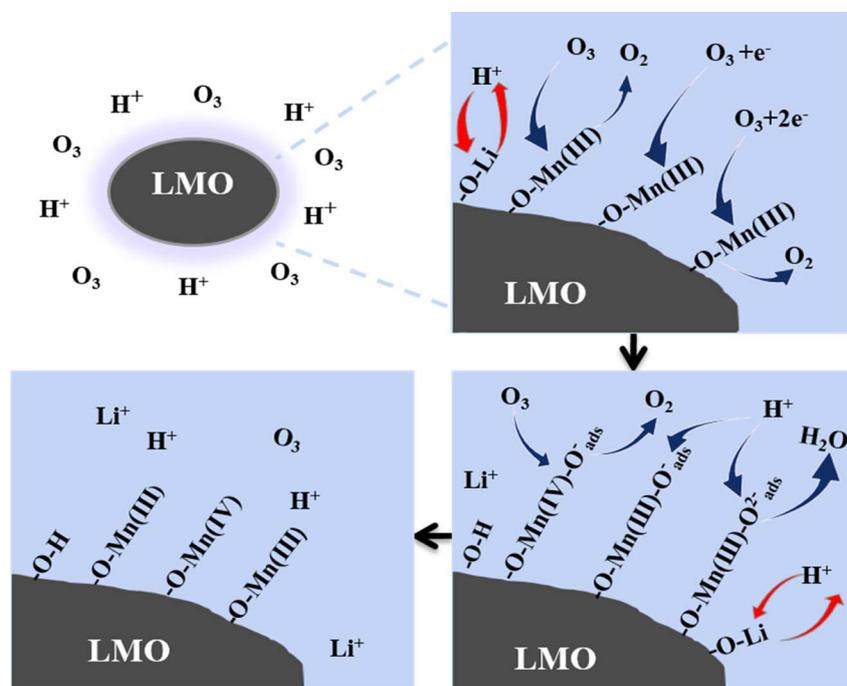
Fig. 8 Mechanism of the Li<sup>+</sup> extraction process using the HCl-O<sub>3</sub> eluent.
