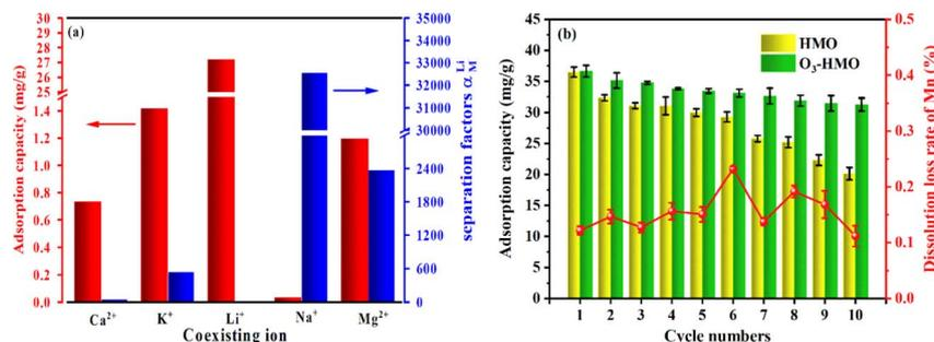
Fig. 11 Recovery of Li<sup>+</sup> from artificial brine via O<sub>3</sub>-HMO: (a) adsorption selectivity towards Li<sup>+</sup>, Na<sup>+</sup>, K<sup>+</sup>, Mg<sup>2+</sup> and Ca<sup>2+</sup>; (b) dissolution loss of Mn and Li<sup>+</sup> adsorption capacity in the cycling process.
