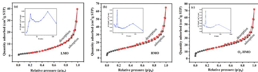
Fig. 4 Nitrogen adsorption–desorption isotherms and pore volume distribution insets: (a) LMO, (b) HMO and (c) O<sub>3</sub>-HMO.
