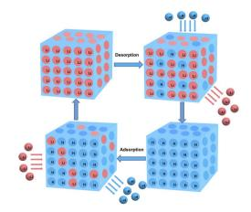
Fig. 1 Schematic diagram of the cyclic application of ion sieves.
