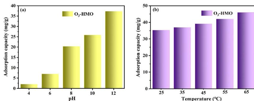
Fig. 9 Effects of different conditions on the adsorption capacity of  $O_3$ -HMO: (a) pH ( $C_{Li^+} = 100 \text{ mg L}^{-1}$ ,  $T = 25^\circ\text{C}$ ), (b) temperature ( $C_{Li^+} = 100 \text{ mg L}^{-1}$ ,  $pH = 11.5$ ).
