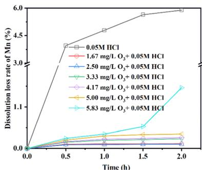
Fig. 6 The MDL of LMO under 0.05 mol L<sup>-1</sup> HCl + R mg L<sup>-1</sup> O<sub>3</sub> (R = 0, 1.67, 2.50, 3.33, 4.17, 5.00, and 5.83).
