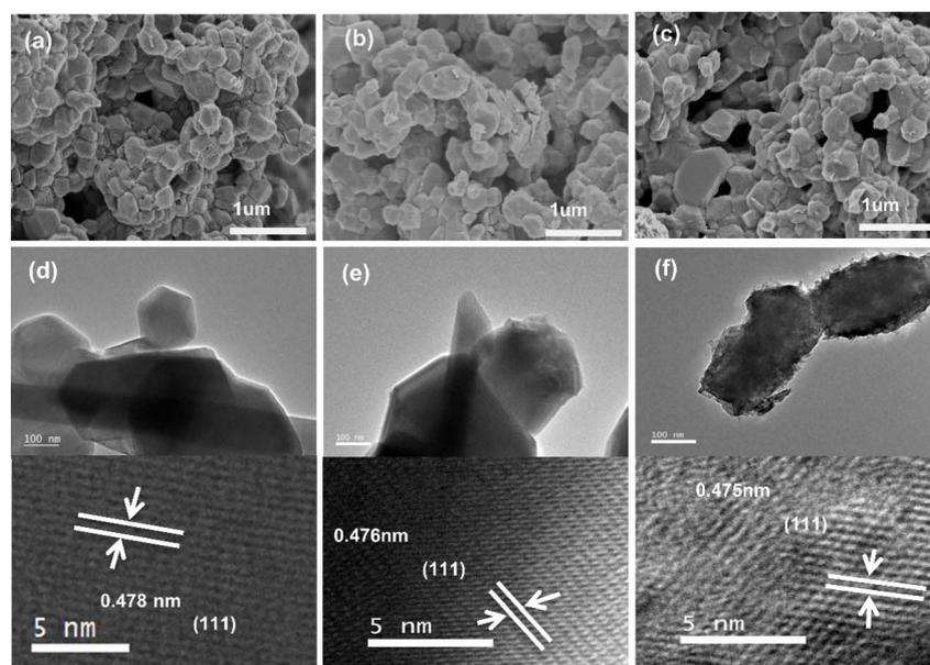
Fig. 3 SEM images of (a) LMO, (b) HMO and (c) O<sub>3</sub>-HMO; TEM images of (d) LMO, (e) HMO, and (f) O<sub>3</sub>-HMO.
