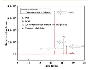
Fig. 7 GC-MS before and after O<sub>3</sub>/Fenton oxidation process.
