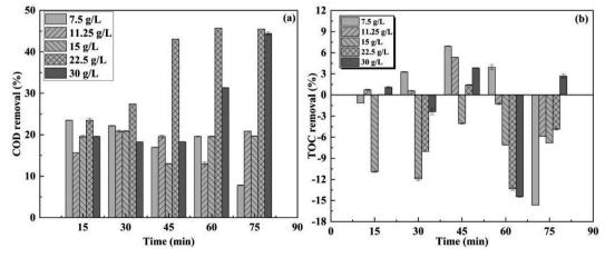
Fig. 3 (a) The COD removal and (b) the TOC removal under different O<sub>3</sub> treatment time.
