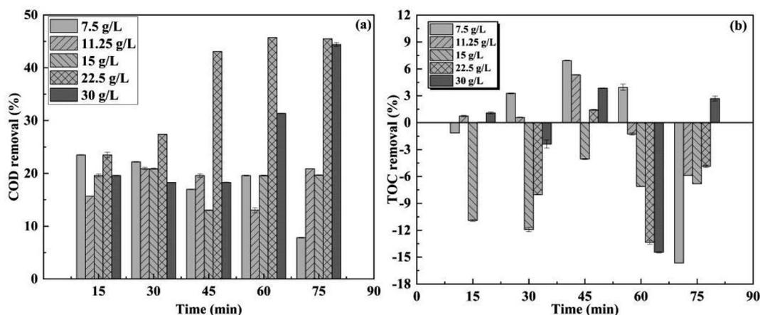
Fig. 3 (a) The COD removal and (b) the TOC removal under different  $\text{O}_3$  treatment time.
