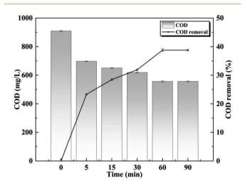
Fig. 2 The COD concentrations and removal with  $O_3$  treatment time.
