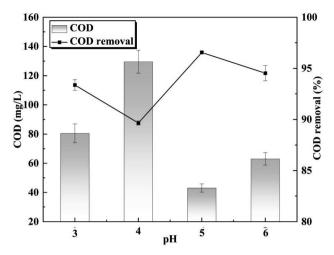
Fig. 6 COD removal during the  $O_3$ /Fenton oxidation process under varying pH conditions.
