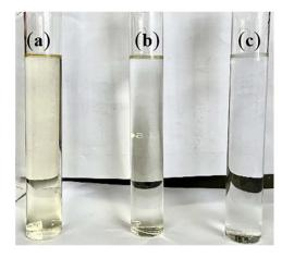
Fig. 8 Different chromatic characteristics of raw APU wastewater (a), wastewater treated by  $O_3/H_2O_2$  process (b), wastewater treated by  $O_3/F_2O_2$  process (c).
