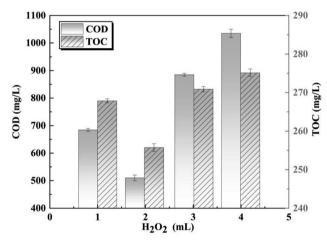
Fig. 4 COD and TOC concentration at different  $H_2O_2$  dosages under  $O_3/H_2O_2$  oxidation process.
