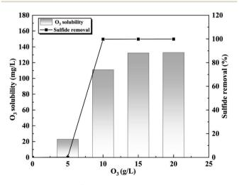
Fig. 1 The solubility of  $O_3$  in water and sulfide removal under different  $O_3$  concentration.
