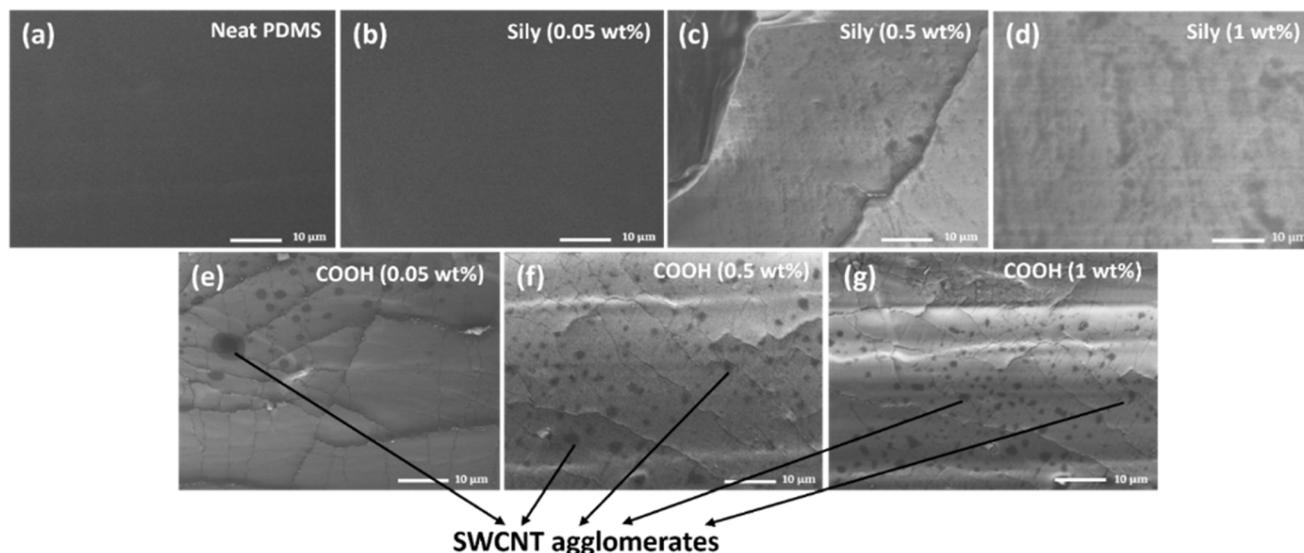
**Fig. 2** Cross-sectional FESEM analysis of the test structures: (a) neat PDMS, (b) PDMS–SWCNT (sily, 0.05 wt%), (c) PDMS–SWCNT (sily, 0.5 wt%), (d) PDMS–SWCNT (sily, 1 wt%) (e) PDMS–SWCNT (COOH, 0.05 wt%), (f) PDMS–SWCNT (COOH, 0.5 wt%), (g) PDMS–SWCNT (COOH, 1 wt%).
