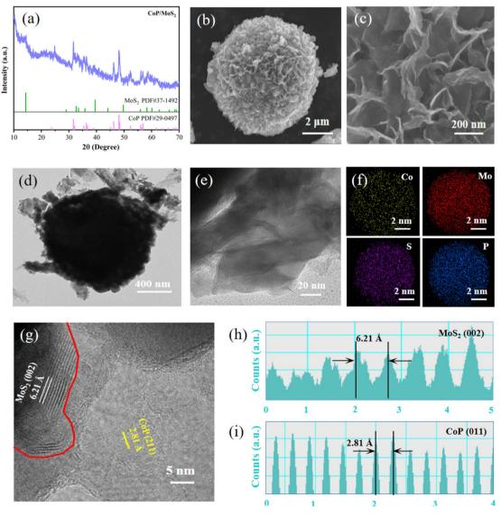
Fig. 1 (a) XRD patterns of CoP/MoS<sub>2</sub>, (b and c) different magnifications of SEM images for CoP/MoS<sub>2</sub>, (d and e) different magnifications of CoP/MoS<sub>2</sub> TEM images, (f) elemental mapping images of CoP/MoS<sub>2</sub>, (g) HRTEM images for CoP/MoS<sub>2</sub>, (h and i) CoP(011) and MoS<sub>2</sub>(002) interplanar spacing.
