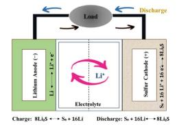
Fig. 2 Basic assembly of lithium sulfur battery
