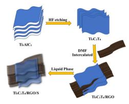
Fig. 11 Depiction of MXene/reduced graphene for trapping sulfur and polysulfides.
