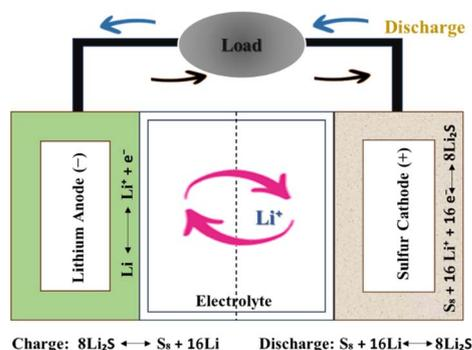
Fig. 2 Basic assembly of lithium sulfur battery.
