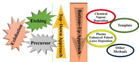
Fig. 4 Different methods for the synthesis of MXene.
