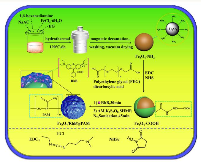
Fig. 1 Schematic illustration of the preparation process of Fe<sub>3</sub>O<sub>4</sub>/RhB@PAM sensors.
