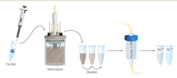
Fig. 3 Schematic of the proposed purification method using Dowex 1-X8 resin packed column.
