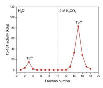
Fig. 5 Elution curve of tracer spiked and electrolysed Tb<sup>4+</sup> solution using a Dowex 1-X8 resin filled cartridge ( $\phi$ : 1 cm, h: 2.5 cm, BV: 2 mL). Feed: 0.4 mL of a solution containing 0.018 mol L<sup>-1</sup> Tb<sup>3+</sup>/Tb<sup>4+</sup> in 1 mol L<sup>-1</sup> K<sub>2</sub>CO<sub>3</sub> solution (pH  $\approx$  12). The vertical dashed line denotes the change of mobile phase from water to 2 mol L<sup>-1</sup> K<sub>2</sub>CO<sub>3</sub>. Flow rate: 0.3 mL min<sup>-1</sup>.
