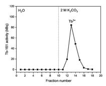
Fig. 4 Elution curve of tracer spiked Tb<sup>3+</sup> solution using a Dowex 1-X8 resin filled cartridge ( $\phi$ : 1 cm, h: 2.5 cm, BV: 2 mL). Feed: 0.4 mL of a solution containing 0.018 mol L<sup>-1</sup> Tb<sup>3+</sup> in 1 mol L<sup>-1</sup> K<sub>2</sub>CO<sub>3</sub> solution (pH  $\approx$  12). The vertical dashed line denotes the change of mobile phase from water to 2 mol L<sup>-1</sup> K<sub>2</sub>CO<sub>3</sub>. Flow rate: 0.3 mL min<sup>-1</sup>.
