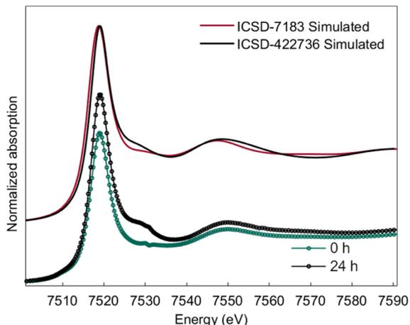
Fig. 9 Simulated  $L_3$ -edge spectra for reference structures ICSD-7183 and ICSD-422736 and comparison with experimental XANES traces of 0 h and 24 h electrolysis.
