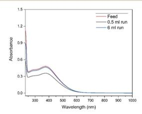
Fig. 1 UV-Vis absorption spectra of the fractions collected at different feed volumes of  $0.07 \, \text{mol L}^{-1} \, \text{Tb}^{4+}$  in 4 mol  $L^{-1} \, \text{K}_2 \text{CO}_3$  solution at pH = 14. Electrolysis was performed at constant potential +1.3 V vs. Ag/AgCl for 3 h. The formation of Tb(v) was followed by the absorbance peak at 365 nm. Blank carbonate solution was used as the reference sample for baseline correction. The cell path length was 1 mm.
