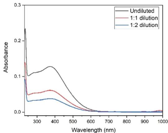
Fig. 2 UV-Vis absorption spectra of the undiluted  $0.07 \text{ mol L}^{-1} \text{ Tb}^{4+}$  in  $4 \text{ mol L}^{-1} \text{ K}_2\text{CO}_3$  solution at  $\text{pH} = 14$ , 1 : 1 (v/v) dilution and 1 : 2 (v/v) dilution. Electrolysis was performed on the undiluted sample at constant potential  $+1.3 \text{ V}$  vs.  $\text{Ag}/\text{AgCl}$  during 30 min. Blank carbonate solution was used as the reference sample for baseline correction. The path length of the quartz cuvette was 1 mm.
