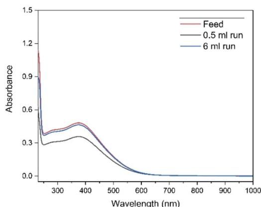
Fig. 1 UV-Vis absorption spectra of the fractions collected at different feed volumes of 0.07 mol L<sup>-1</sup> Tb<sup>4+</sup> in 4 mol L<sup>-1</sup> K<sub>2</sub>CO<sub>3</sub> solution at pH = 14. Electrolysis was performed at constant potential +1.3 V vs. Ag/AgCl for 3 h. The formation of Tb(IV) was followed by the absorbance peak at 365 nm. Blank carbonate solution was used as the reference sample for baseline correction. The cell path length was 1 mm.
