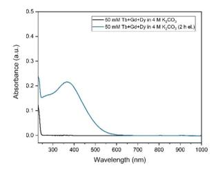
Fig. 6 UV–Vis absorption spectra of 0.05 mol L $^{-1}$ Tb $^{3+}$ , 0.05 mol L $^{-1}$ Gd $^{3+}$  and 0.05 mol L $^{-1}$ Dy $^{3+}$  in 4 mol L $^{-1}$ K $_2$ CO $_3$  at pH = 14, before and after the electrolysis. Electrolysis was performed at constant potential +1.3 V vs. Ag/AgCl for 2 h. The formation of Tb $^{4+}$  was followed by the absorbance peak at 365 nm. Blank carbonate solution was used as the reference sample for baseline correction. The path length was 1 mm.
