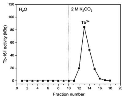
Fig. 4 Elution curve of tracer spiked  $\text{Tb}^{3+}$  solution using a Dowex 1-X8 resin filled cartridge ( $\phi$ : 1 cm,  $h$ : 2.5 cm, BV: 2 mL). Feed: 0.4 mL of a solution containing  $0.018 \text{ mol L}^{-1} \text{ Tb}^{3+}$  in  $1 \text{ mol L}^{-1} \text{ K}_2\text{CO}_3$  solution ( $\text{pH} \approx 12$ ). The vertical dashed line denotes the change of mobile phase from water to  $2 \text{ mol L}^{-1} \text{ K}_2\text{CO}_3$ . Flow rate:  $0.3 \text{ mL min}^{-1}$ .
