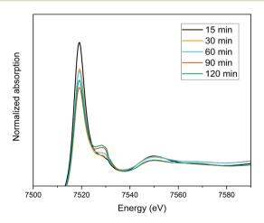
Fig. 8 Normalized XANES spectra of the oxidation of 0.07 mol  $L^{-1}$  $\text{Tb}^{3+}$  in a 4 mol  $\text{L}^{-1}$  K<sub>2</sub>CO<sub>3</sub> solution as a function of time (15 min-120 min).
