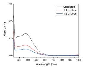
Fig. 2 UV–Vis absorption spectra of the undiluted 0.07 mol  $L^{-1}$  Tb<sup>4+</sup> in 4 mol  $L^{-1}$  K<sub>2</sub>CO<sub>3</sub> solution at pH = 14, 1:1 (v/v) dilution and 1:2 (v/v) dilution. Electrolysis was performed on the undiluted sample at constant potential +1.3 V vs. Ag/AgCl during 30 min. Blank carbonate solution was used as the reference sample for baseline correction. The path length of the quartz cuvette was 1 mm.
