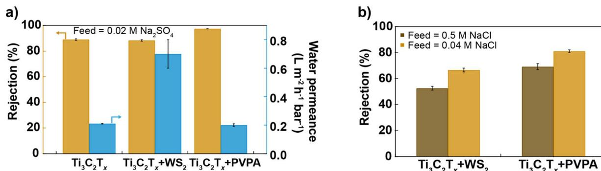
Fig. 4 Effect of hydrophilicity and surface charge modulation on the performance of MXene-based membranes. Comparison of performance of Ti<sub>3</sub>C<sub>2</sub>T<sub>x</sub>-based membranes in the cross-flow filtration system for 0.02 M Na<sub>2</sub>SO<sub>4</sub> (a), and 0.04 M and 0.5 M NaCl (b). Error bars represent the standard deviations of at least three replicates.
