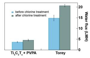
Fig. 5 Comparison of chlorine-resistance test of our Ti<sub>3</sub>C<sub>2</sub>T<sub>x</sub> + PVPA membranes Toray Flat sheet membranes, UTC-82V PA RO membrane (Sterlitech). Membranes (not treated with NaOCl solution and treated with 4000 ppmh of NaOCl solution) were tested in a cross-flow system with 0.02 M Na<sub>2</sub>SO<sub>4</sub> as feed solution. Error bars represent the standard deviations of at least three replicates
