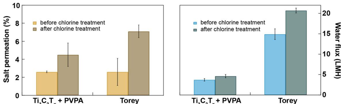
Fig. 5 Comparison of chlorine-resistance test of our  $\text{Ti}_3\text{C}_2\text{T}_x$  + PVPA membranes Toray Flat sheet membranes, UTC-82V PA RO membrane (Sterlitech). Membranes (not treated with NaOCl solution and treated with 4000 ppmh of NaOCl solution) were tested in a cross-flow system with 0.02 M  $\text{Na}_2\text{SO}_4$  as feed solution. Error bars represent the standard deviations of at least three replicates.
