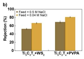
Fig. 4 Effect of hydrophilicity and surface charge modulation on the performance of MXene-based membranes. Comparison of performance of  $Ti_3C_2T_x$ -based membranes in the cross-flow filtration system for 0.02 M  $Na_2SO_4$  (a), and 0.04 M and 0.5 M NaCl (b). Error bars represent the standard deviations of at least three replicates.
