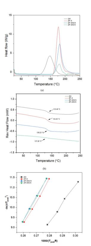
Fig. 4 The DSC plots for epoxy compositions with different promoters: (a) change in  $T_{\rm peak}$  (b) glass transition temperature ( $T_{\rm g}$ ), and (c) Kissinger plots of activation energy.
