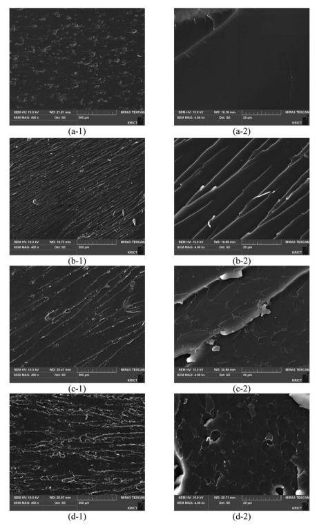
Fig. 7 SEM images of the fractured surfaces of Izod test specimens for different promoters: (a1-a2) 2MI, (b1-b2) ZIF-8, (c1-c2) ZIF-8/GCN, and (d1-d2) ZIF-8/SCN.
