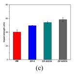
Fig. 6 Mechanical properties of epoxy compositions with different promoters: (a) tensile (MPa), (b) flexural (MPa), and (c) impact (J  $m^{-1}$ ) strenaths
