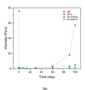
Fig. 8 The plot of change in viscosity over time for different promoters in the curing system at (a) 40 °C and (b) 60 °C.
