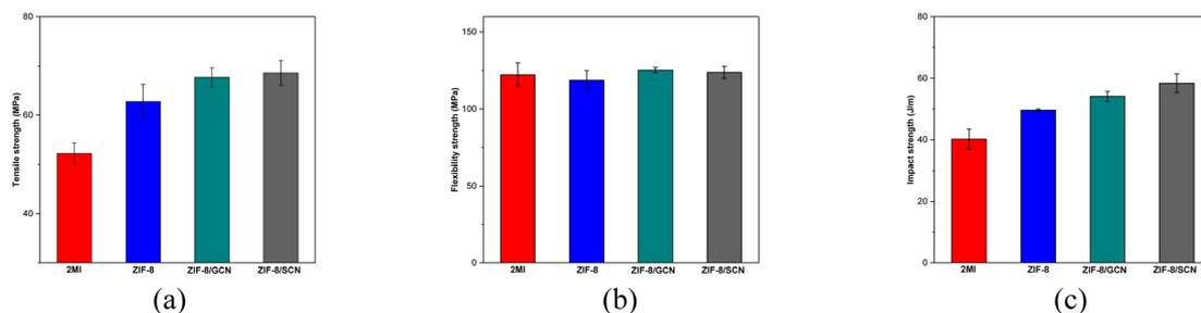
Fig. 6 Mechanical properties of epoxy compositions with different promoters: (a) tensile (MPa), (b) flexural (MPa), and (c) impact (J m<sup>-1</sup>) strengths.
