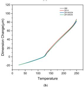
Fig. 5 (a) DMA and (b) TMA data for epoxy compositions with different promoters.
