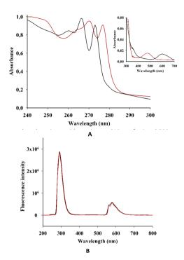
Fig. 4 (A) EAS and (B) fluorescent spectra ( $\lambda_{exc}=250$  nm) of I (black) and II (red) in acetonitrile. (Inset in A) EAS of I and II in the long wave area.
