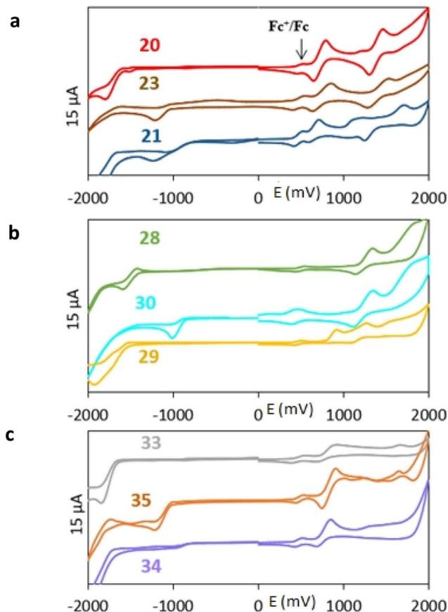
Fig. 3 Cyclic voltammograms of all D- $\pi$ -A derivatives (1 mM) – (a) the compounds with the 2,5-diphenylthiophene bridge; (b) the compounds with the terphenyl bridge; (c) the compounds with the terphenyl bridge, all on the platinum electrode in dichloromethane with the basic electrolyte of 0.1 M ([NBu<sub>4</sub>][PF<sub>6</sub>]). The potential scale corresponds to the Ag/AgCl reference electrode.
