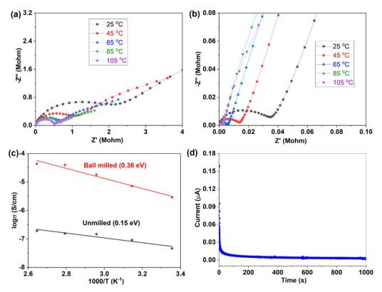
Fig. 4 Variable temperature EIS of 500 °C samples before (a) and after (b) ball milling, (c) Arrhenius plots of 500 °C samples before and after ball milling, (d) DC polarization curve of 500 °C sample after ball milling.
