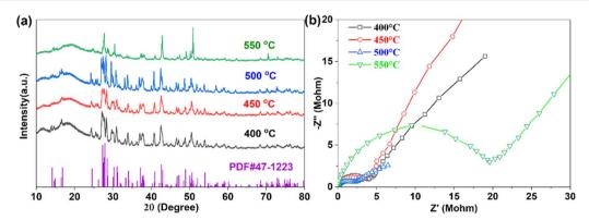
Fig. 1 XRD pattern (a) and EIS (b) of Na<sub>3</sub>YBr<sub>6</sub> sintered at different temperatures.
