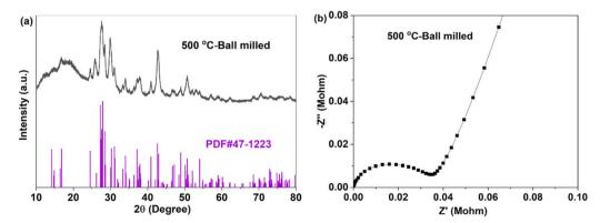
Fig. 3 XRD pattern (a) and EIS (b) of Na<sub>3</sub>YBr<sub>6</sub> sintered at 500 °C and ball milled at 500 rpm for 10 h.
