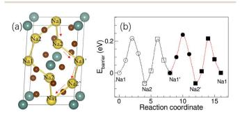
Fig. 5 (a) The structure of  $Na_3YBr_6$  and diffusion path of  $Na^+$ , (b) the migration energy barrier of  $Na^+$  in the  $Na_3YBr_6$ .
