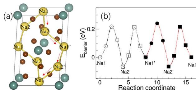
Fig. 5 (a) The structure of Na<sub>3</sub>YBr<sub>6</sub> and diffusion path of Na<sup>+</sup>, (b) the migration energy barrier of Na<sup>+</sup> in the Na<sub>3</sub>YBr<sub>6</sub>.
