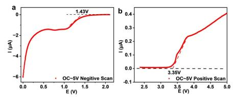
Fig. 6 Linear scanning voltammetry of a Na|Na<sub>2.9</sub>PS<sub>3.9</sub>Cl<sub>0.1</sub>|Na<sub>3</sub>YBr<sub>6</sub> + C cell.
