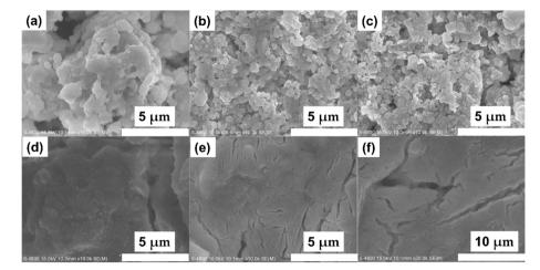
Fig. 2 SEM images of Na<sub>3</sub>YBr<sub>6</sub> sintered at 400 °C (a), 450 °C (b), 500 °C (c), 550 °C (d), and Na<sub>3</sub>YBr<sub>6</sub> ball milled at 500 rpm after sintering at 500 °C (e and f).
