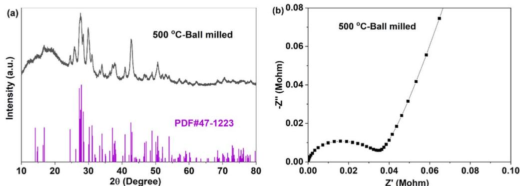
Fig. 3 XRD pattern (a) and EIS (b) of  $\text{Na}_3\text{YBr}_6$  sintered at 500 °C and ball milled at 500 rpm for 10 h.
