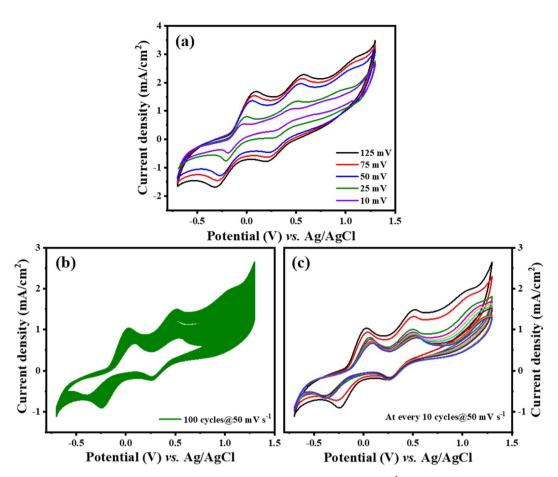
Fig. 6 (a)  $Ti_3C_2T_x$ -PTh at various scan rates (b) and (c) stability test of  $Ti_3C_2T_x$ -PTh at 50 mV s<sup>-1</sup> for 100 cycles and plotted at every 10 cycles.
