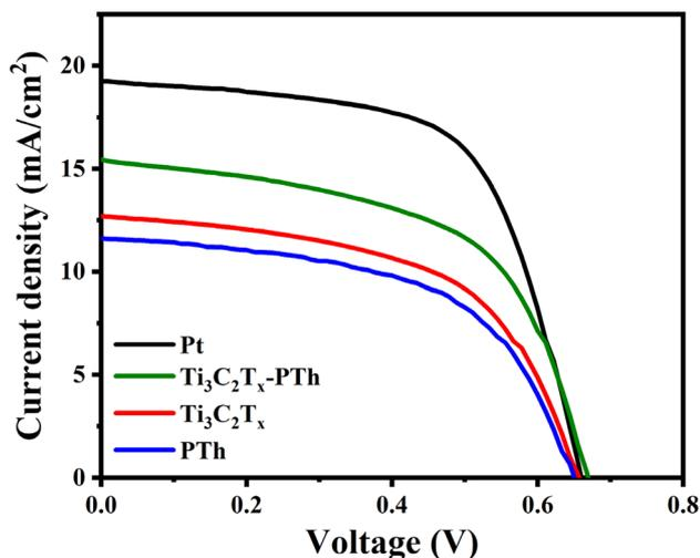
**Fig. 8**  $J$ - $V$  photocurrent density-voltage curves of DSSC fabricated with Pt,  $\text{Ti}_3\text{C}_2\text{T}_x$ , PTh, and  $\text{Ti}_3\text{C}_2\text{T}_x$ -PTh CEs.
