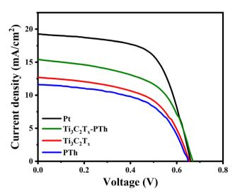
Fig. 8 J-V photocurrent density-voltage curves of DSSC fabricated with Pt,  $Ti_3C_2T_v$ , PTh, and  $Ti_3C_2T_v$ -PTh CEs.
