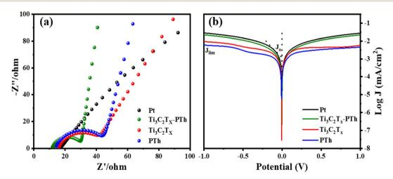
Fig. 7 (a) Electrochemical impedance spectra of Pt,  $Ti_3C_2T_x$ , PTh and  $Ti_3C_2T_x$ -PTh CEs made from the symmetrical cell (b) Tafel polarisation of Pt,  $Ti_3C_2T_x$ . PTh and  $Ti_3C_2T_x$ -PTh CEs.
