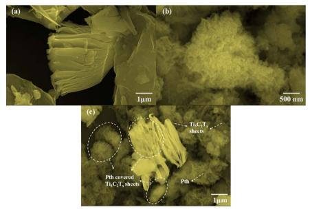
Fig. 3 SEM images of (a) pristine  $Ti_3C_2T_x$ , (b) pristine Pth, and (c)  $Ti_3C_2T_x$ -Pth.
