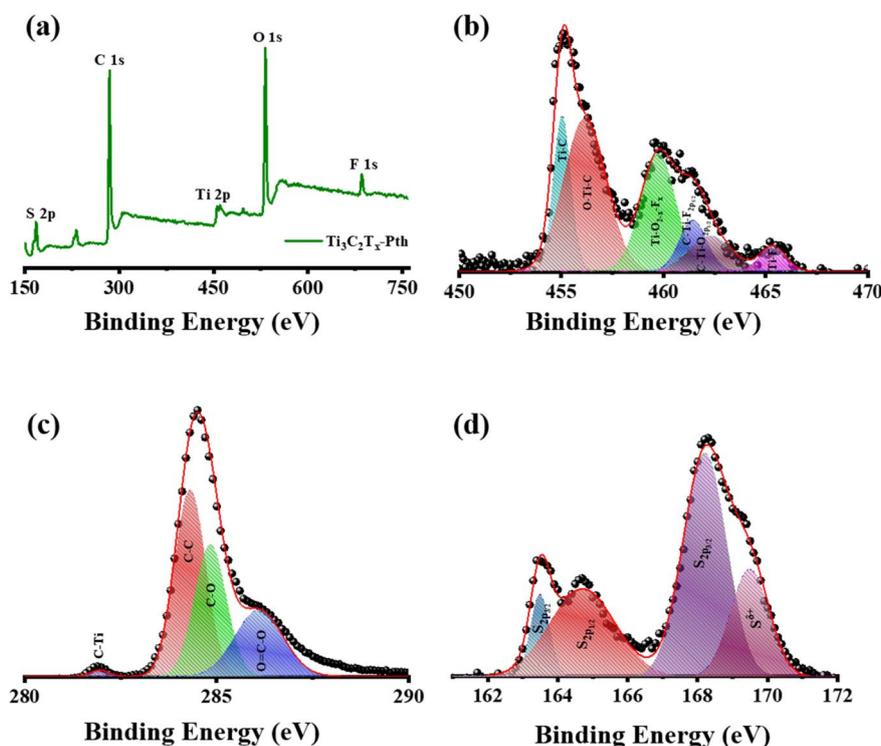
Fig. 4 (a) XPS survey spectrum of Ti<sub>3</sub>C<sub>2</sub>T<sub>x</sub>-Pth, and XPS patterns of (b) Ti 2p, (c) C 1s, and (d) S 1s.
