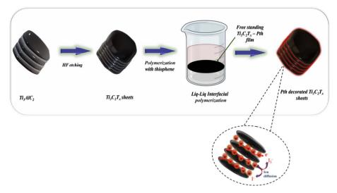
Fig. 1 A schematic representation of the synthesis of Ti<sub>3</sub>C<sub>2</sub>T<sub>x</sub>-Pth.
