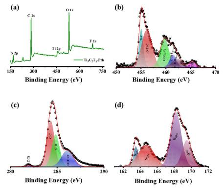
Fig. 4 (a) XPS survey spectrum of  $Ti_7C_2T_x$ -Pth, and XPS patterns of (b) Ti 2p, (c) C 1s, and (d) S 1s.
