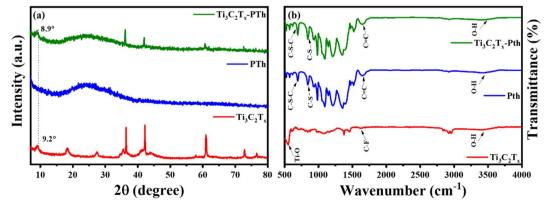
Fig. 2 (a) XRD patterns and (b) FT-IR spectra of Ti<sub>3</sub>C<sub>2</sub>T<sub>x</sub>, Pth, and Ti<sub>3</sub>C<sub>2</sub>T<sub>x</sub>-Pth.
