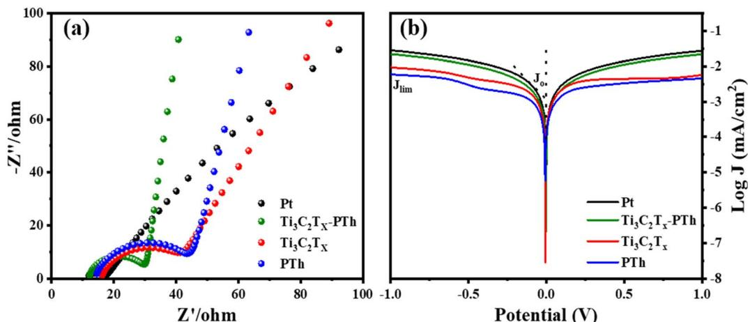
Fig. 7 (a) Electrochemical impedance spectra of Pt,  $\text{Ti}_3\text{C}_2\text{T}_x$ , PTh and  $\text{Ti}_3\text{C}_2\text{T}_x\text{-PTh}$  CE made from the symmetrical cell (b) Tafel polarisation of Pt,  $\text{Ti}_3\text{C}_2\text{T}_x$ , PTh and  $\text{Ti}_3\text{C}_2\text{T}_x\text{-PTh}$  CE.
