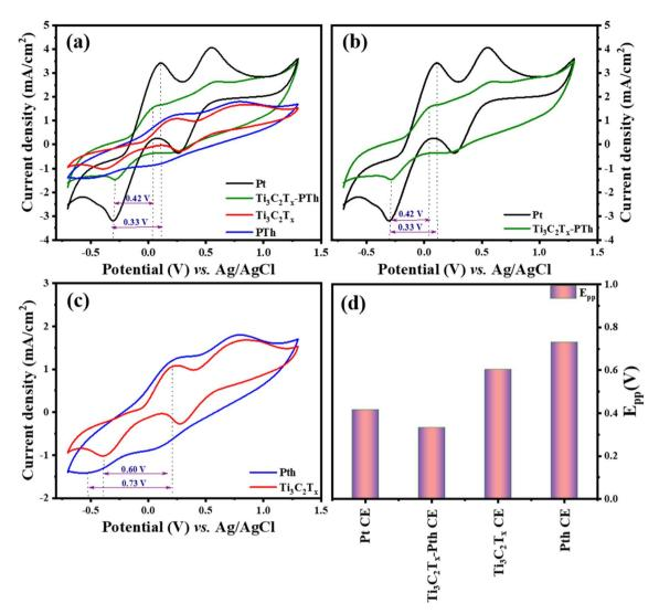
Fig. 5 Cyclic voltammograms of (a) Pt,  $Ti_3C_2T_x$ , Pth,  $Ti_3C_2T_x$ -Pth at 50 mV s<sup>-1</sup> scan rate (b-d) comparison of cyclic voltammograms Pt and  $Ti_3C_2T_x$ -Pth CEs,  $Ti_3C_2T_x$  and Pth CEs, and overall  $E_{pp}$  comparison of Pt,  $Ti_3C_2T_x$ , Pth,  $Ti_3C_2T_x$ -Pth CEs.
