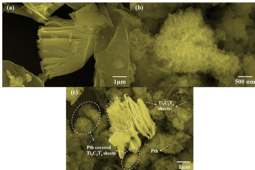
Fig. 3 SEM images of (a) pristine Ti<sub>3</sub>C<sub>2</sub>T<sub>x</sub>, (b) pristine Pth, and (c) Ti<sub>3</sub>C<sub>2</sub>T<sub>x</sub>-Pth.
