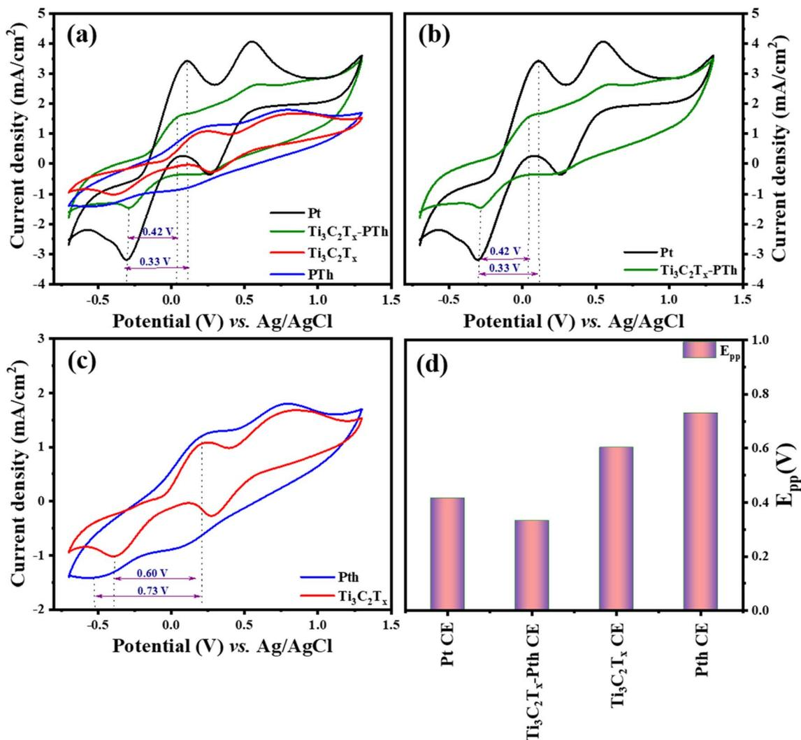
Fig. 5 Cyclic voltammograms of (a) Pt, Ti<sub>3</sub>C<sub>2</sub>T<sub>x</sub>, Pth, Ti<sub>3</sub>C<sub>2</sub>T<sub>x</sub>-Pth at 50 mV s<sup>-1</sup> scan rate (b–d) comparison of cyclic voltammograms Pt and Ti<sub>3</sub>C<sub>2</sub>T<sub>x</sub>-Pth CEs, Ti<sub>3</sub>C<sub>2</sub>T<sub>x</sub> and Pth CEs, and overall E<sub>pp</sub> comparison of Pt, Ti<sub>3</sub>C<sub>2</sub>T<sub>x</sub>, Pth, Ti<sub>3</sub>C<sub>2</sub>T<sub>x</sub>-Pth CEs.
