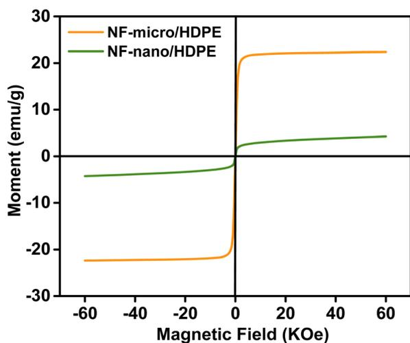
Fig. 13 Hysteresis loops of magnetic composite materials.
