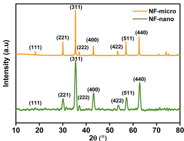
Fig. 2 XRD pattern of NF-micro and NF-nano powder.
