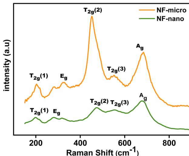
Fig. 3 Raman spectra of NF-micro and NF-nano.
