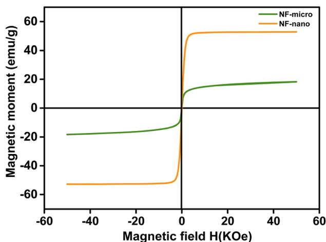
Fig. 7 Magnetic properties of NiFe<sub>2</sub>O<sub>4</sub> nano and micro particles.
