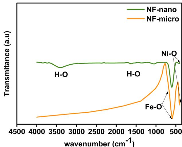
Fig. 4 FTIR spectra of NF-micro and NF-nano.
