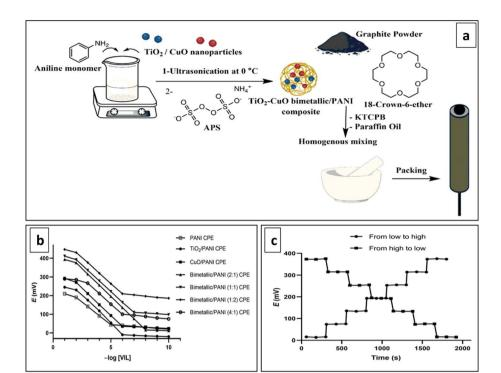
Fig. 10 (a) Diagram outlining the fabrication process of the electrode with  $TiO_2$ -CuO bimetallic/PANI nanocomposite transducer, (b) potentiometric responses and (c) dynamic response time of the electrode. Reproduced with permission. <sup>149</sup> Copyright 2023, MDPI, Basel, Switzerland.
