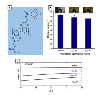
Fig. 12 (a) Molecular structure of P(EDOTF-EDOT-TEMPO), (b) water contact angles and (c) potential stability of conditioned SC-ISEs that SCs were pre-polarized at different potentials. Reproduced with permission.<sup>34</sup> Copyright 2023, Elsevier.
