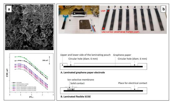
Fig. 9 (a) SEM image of PANI NFs-Cl: MWCNTs composite (upper) and potentiometric responses of the SC-ISEs (lower). Reproduced with permission. Copyright 2022, MDPI, Basel, Switzerland. (b) Required equipment for the fabrication process, laminated graphene paper electrodes (upper) and schematic side view of the flexible SC-ISEs (lower). Reproduced with permission. Copyright 2021, Elsevier.
