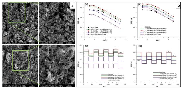
Fig. 6 (a) SEM micrographs of PANI NFs-Cl (upper) and PANI NFs-NO<sub>3</sub> (lower) and (b) ISE performances. Reproduced with permission.<sup>53</sup> Copyright 2021, Springer.
