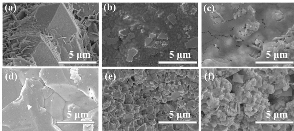
Fig. 2 (a–c) Top-view SEM images of perovskite about  $n = \infty$ ,  $n = 10$ , and  $n = 6$ , respectively; (d–f) cross-sectional SEM images of perovskite about  $n = \infty$ ,  $n = 10$ , and  $n = 6$ , respectively.
