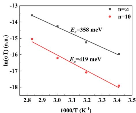
Fig. 7 Temperature-dependent conductivity test.
