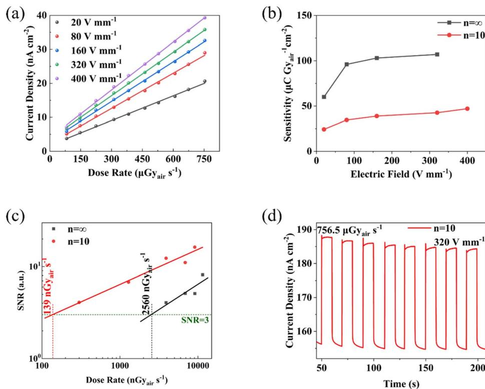
**Fig. 8** (a) Photocurrent density–dose curves of the  $n = 10$  under different electric field; (b) summary of the sensitivities of  $n = 10$  and  $n = \infty$  at different electric fields; (c) signal-to-noise ratio versus X-ray dose rate for  $n = 10$  and  $n = \infty$ , with the limit of detection obtained through linear fitting; (d) the cycle stability of  $n = 10$  device at  $320 \text{ V mm}^{-1}$  electric field (8 consecutive on–off cycles).
