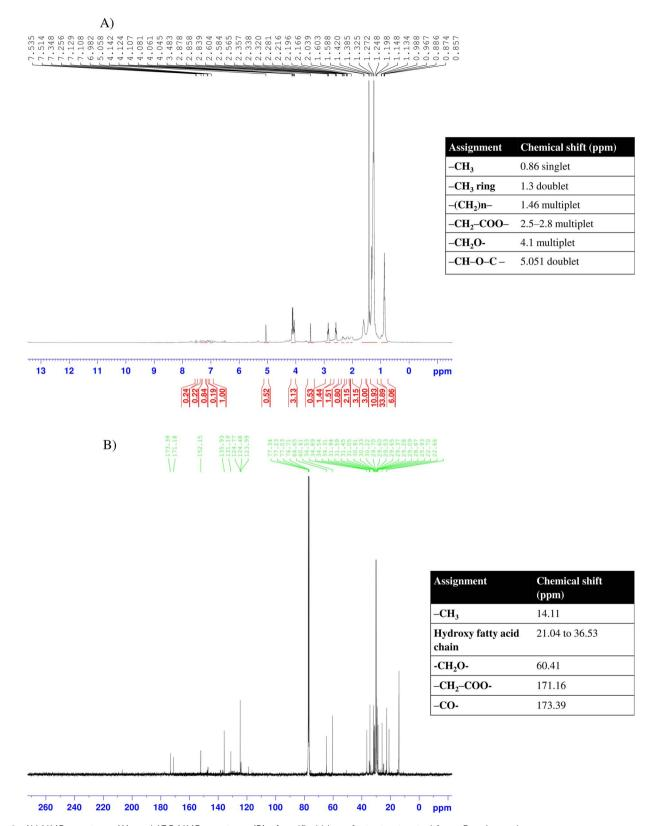
Fig. 6 1H NMR spectrum (A), and 13C NMR spectrum (B) of purified biosurfactant extracted from B. velezensis.
