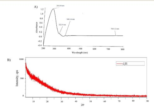
Fig. 9 The optical characteristics of purified biosurfactant exhibiting its UV absorbance at 265.01 nm (A), amorphic structure identified by XRD (B).
