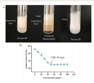
Fig. 11 An observation of foaming and emulsification stability of the isolated rhamnolid in presence of pure tween-20 (commercial surfactant) and tween-80 (commercial emulsifier) (A); the CMC of purified biosurfactant determined by plotting the surface tension against the respective concentrations of the surfactant (B). Here, error bars represent the standard deviations (n = 3).
