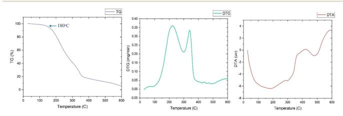
Fig. 10 A graphical illustration showing the thermogravimetric (TG), difference thermo-gravimetric (DTG), and differential thermal analysis (DTA) performed on the extracted biosurfactant produced from S2 strain.
