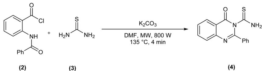
Scheme 1 Microwave-assisted synthesis of 4-oxo-2-phenylquinazoline-3(4H)-carbothioamide.
