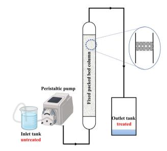
Fig. 2 Schematic representation of packed-bed column setup.
