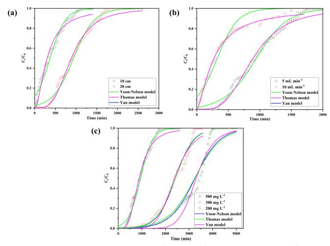
Fig. 16 Effect of (a) packed-bed height (Z: 10–20 cm; Q: 5 mL min<sup>-1</sup>; Z: 500 mg L<sup>-1</sup>), (b) inlet flow rate (Q: 5–10 mL min<sup>-1</sup>; Z: 20 cm;  $C_0$ : 500 mg L<sup>-1</sup>), and (c) inlet Pb<sup>2+</sup> ion concentration ( $C_0$ : 200, 300, and 500 mg L<sup>-1</sup>; Q: 5 mL min<sup>-1</sup>; Z: 20 cm).
