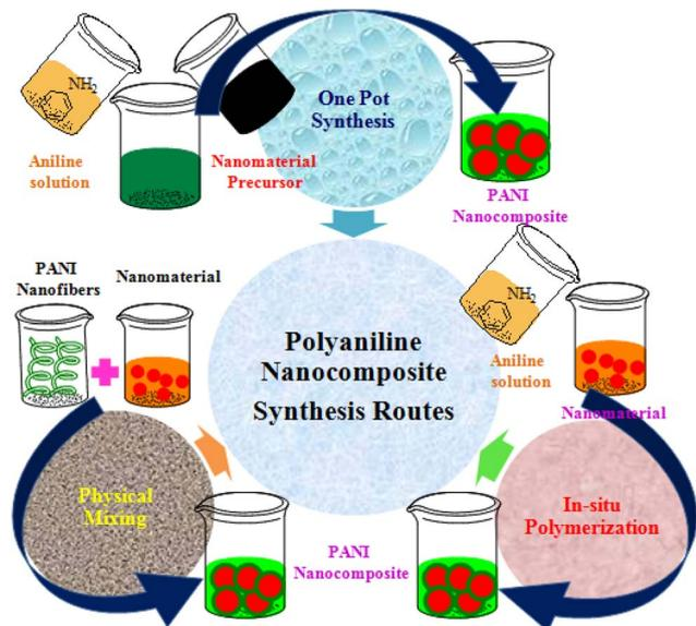
Fig. 2 Polyaniline nanocomposite synthesis routes.
