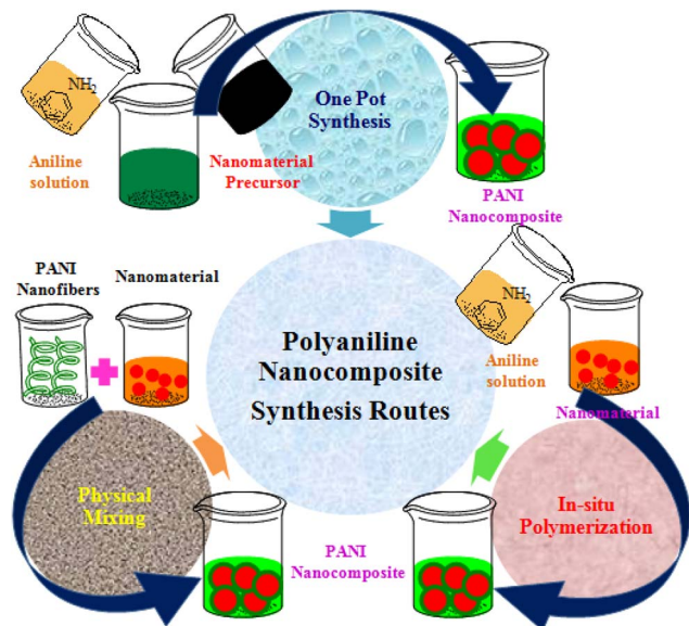
Fig. 2 Polyaniline nanocomposite synthesis routes.
