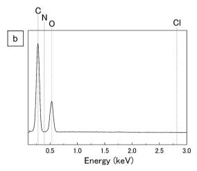
Fig. 6 SEM-EDX analysis on DES-water insoluble portion after heating of ChCl/glucose DES at  $160\,^{\circ}$ C for  $180\,$ min. (a) the SEM image. (b) The EDX spectrum on square area in (a).
