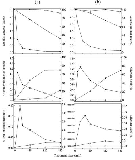
Fig. 5 Residual rate of glucose and the yields of oligomer and 5-HMF, and the amount of each substance during the heating of ChCl/glucose DES (a) and neat glucose (b) at 100 °C (▲), 130 °C (●), and 160 °C (■). The left axis shows the number of moles of each substance, and the right axis shows the yield.
