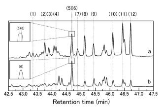
Fig. 4 Total ion chromatograms obtained in the GC-MS analysis of (a) the trimethylsilylated ChCl/glucose DES and (b) the trimethylsilylated glucose after heating at  $130\,^{\circ}$ C for  $180\,$ min.
