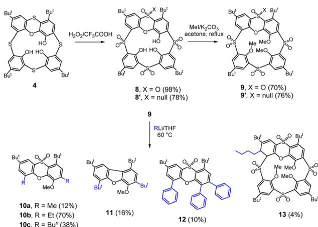
Scheme 3 Cleavage of compound 9 with organolithium compounds.
