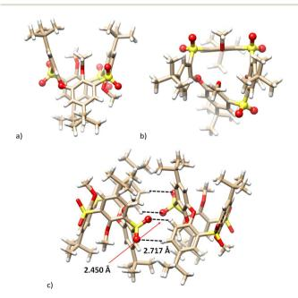
Fig. 5 Single crystal X-ray structure of the compound 15. (a) Side view; (b) top view; bridging moieties shown as balls for better clarity; (c) dimeric motif in the crystal packing showing the  $S=O\cdots H-C(ar)$  intermolecular HB interactions (interacting atoms shown as balls).
