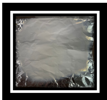
Fig. 2 Fabrication results of HA/PCL/gelatin nanofiber scaffolds.
