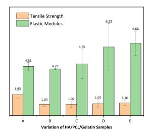
Fig. 7 Ultimate Tensile Strength (UTS) and elastic modulus of HA/PCL/gelatin nanofiber scaffold samples: (A) 50:40:10, (B) 50:30:20, (C) 50:25:25, (D) 50:20:30 and (E) 50:35:15 (in wt%).
