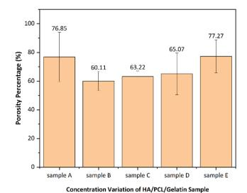
Fig. 5 Graph of porosity test results for HA/PCL/gelatin nanofiber scaffold samples (in wt%): (A) 50:40:10, (B) 50:30:20, (C) 50:25:25, (D) 50:20:30 and (E) 50:35:15.
