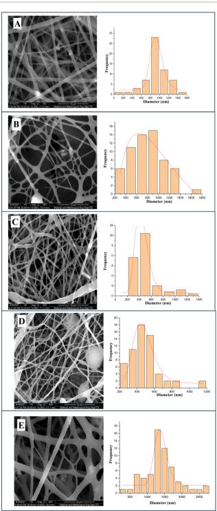
Fig. 4 SEM test results  $-10\,000\times$  magnification and distribution of fiber diameters for HA/PCL/gelatin samples with variations in the ratio of sample (A) 50:40:10 sample (B) 50:30:20 sample (C) 50:25:25 sample (D) 50:20:30 and sample (E) 50:35:15.
