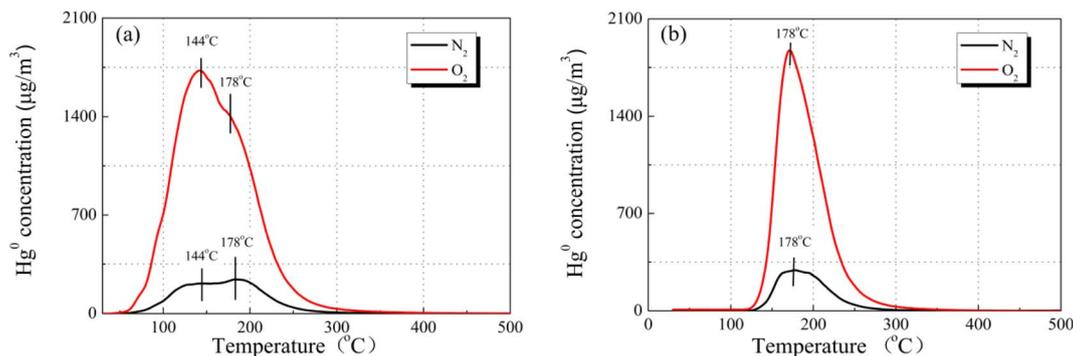
Fig. 8  $\text{Hg}^0$ -TPD patterns of the 12% CuO/AC catalyst after pre-adsorption in an  $\text{N}_2$  or  $\text{O}_2$  atmosphere (a) without  $\text{N}_2$  purge and (b) with  $\text{N}_2$  purge at 120 °C (pre-adsorption reaction conditions: 7%  $\text{O}_2$  and  $\text{N}_2$  as the balance).
