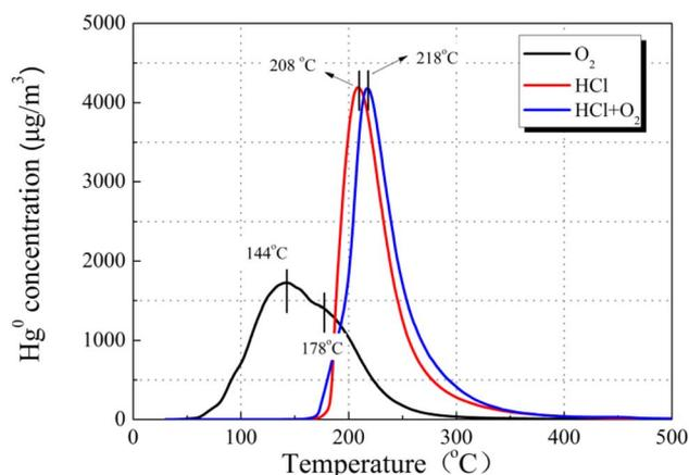
Fig. 14  $\text{Hg}^0$ -TPD patterns of the 12% CuO/AC catalyst after pre-adsorption in HCl at 120 °C (pre-adsorption reaction conditions: 15 ppm of HCl, 7%  $\text{O}_2$ , and  $\text{N}_2$  as the balance).
