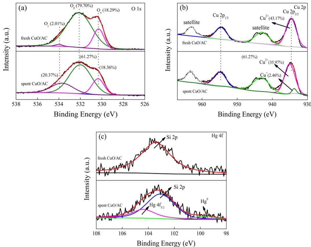
Fig. 6 (a) O 1s, (b) Cu 2p and (c) Hg 4f profiles of fresh AC and spent 12% CuO/AC catalysts.
