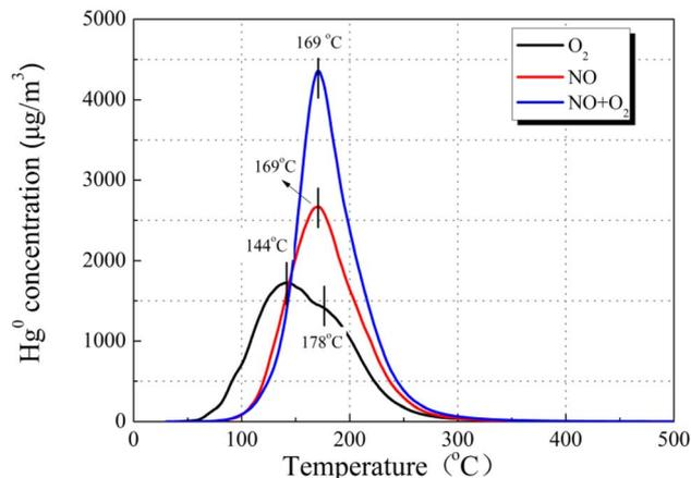
Fig. 12  $\text{Hg}^0$ -TPD patterns of the 12% CuO/AC catalyst after pre-adsorption in NO at 120 °C (pre-adsorption reaction conditions: 500 ppm of NO, 7%  $\text{O}_2$ , and  $\text{N}_2$  as the balance).
