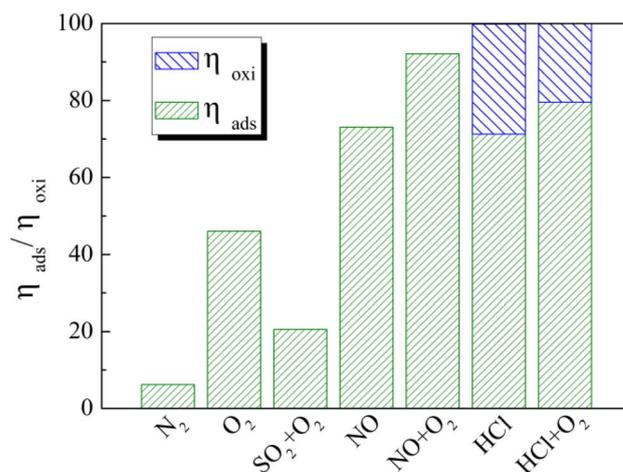
Fig. 15 Effect of individual flue gas components on  $\text{Hg}^0$  adsorption and oxidation over the 12% CuO/AC catalyst at 120 °C.
