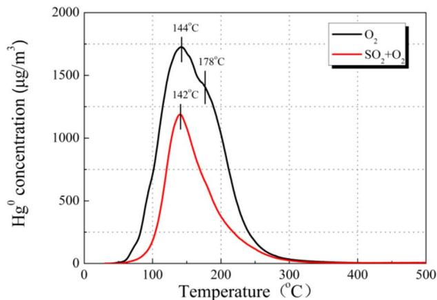
Fig. 10  $\text{Hg}^0$ -TPD patterns of the 12% CuO/AC catalyst after pre-adsorption in  $\text{SO}_2$  at 120 °C (pre-adsorption reaction conditions: 200 ppm of  $\text{SO}_2$ , 7%  $\text{O}_2$ , and  $\text{N}_2$  as the balance).
