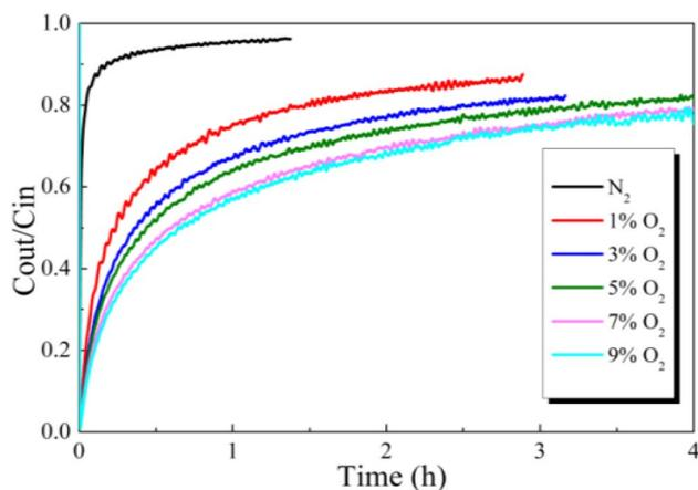
Fig. 7 Effect of O<sub>2</sub> concentration balanced in N<sub>2</sub> on Hg<sup>0</sup> removal over the 12% CuO/AC catalyst at 120 °C.
