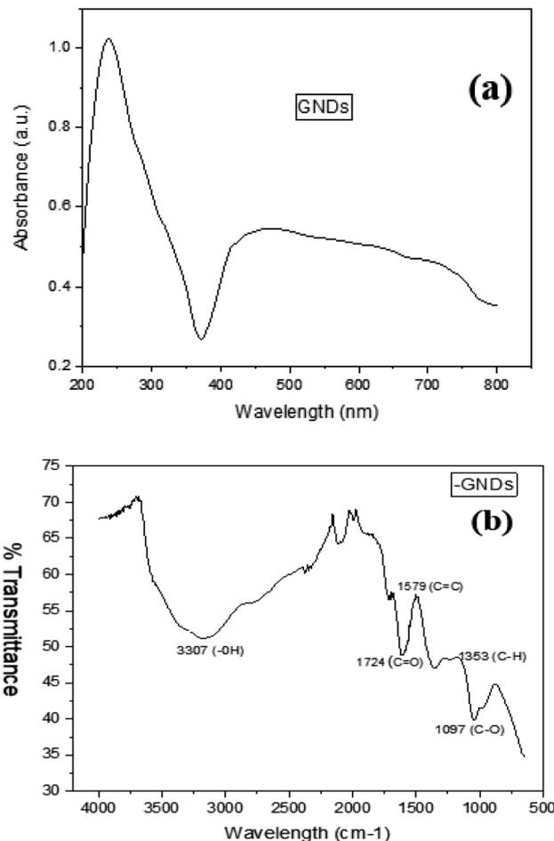
Fig. 2 (a) UV-visible (b) FTIR spectra of GNDs.
