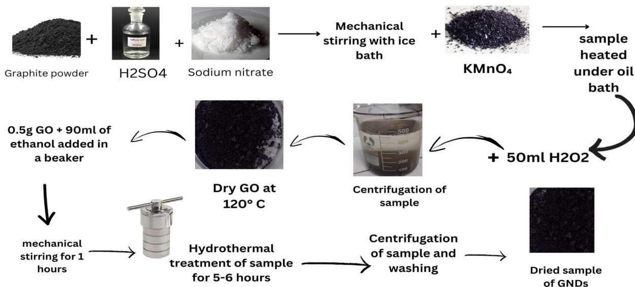
Fig. 1 Schematic diagram showing synthesis of graphene nanodots.
