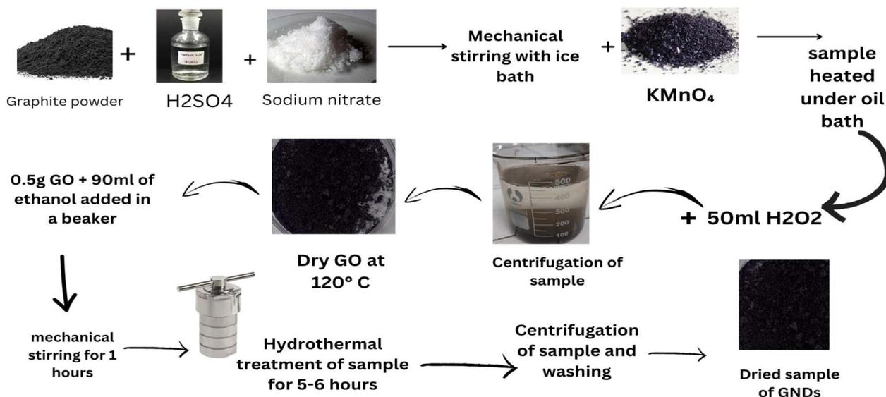
Fig. 1 Schematic diagram showing synthesis of graphene nanodots.
